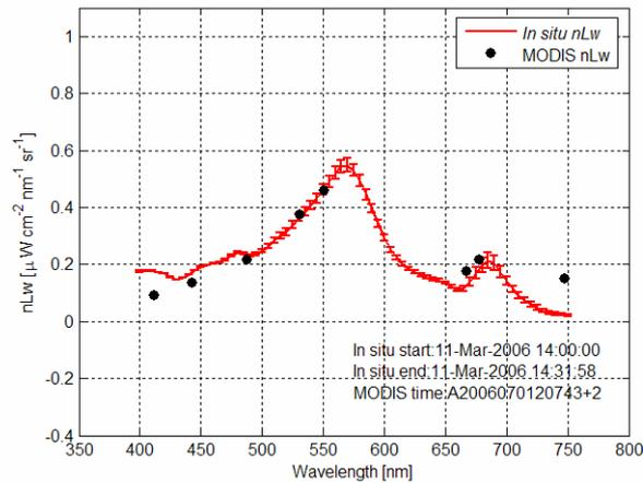
Fig. 5. Comparison of in situ and MODIS-Aqua water-leaving radiance spectra.
