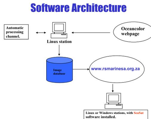
Fig. 1. RS server software architecture
