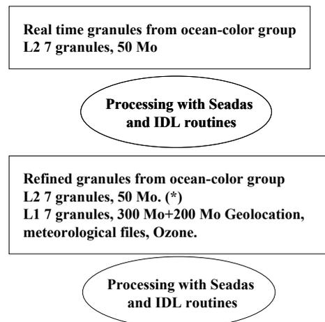
Fig. 2. Processing channels for MODIS data
