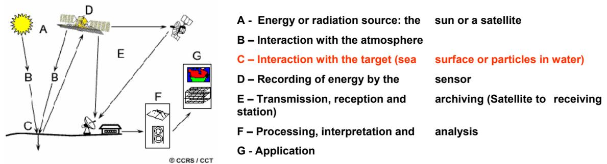
Fig. 3. Processes in satellite remote sensing
