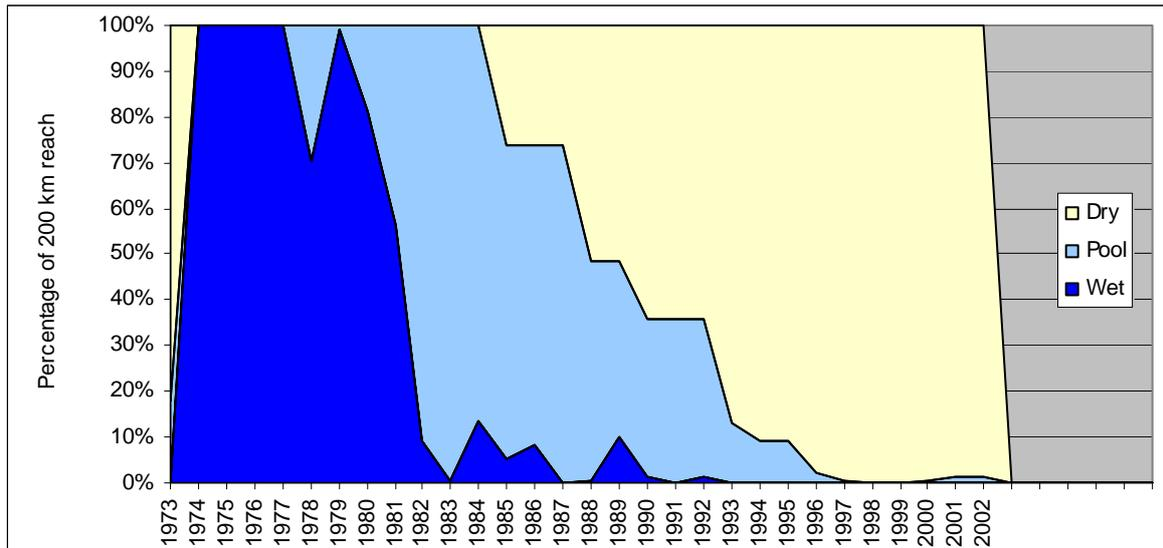
Figure 5-15 : Percentage of the Boteti River study reach that will be inundated (wet); isolated pools (pool) and dry under the Medium Scenario
