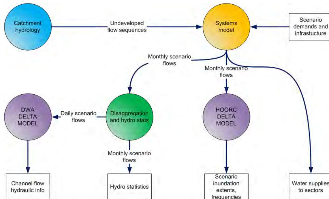
Figure 2-1 : Hydrological Modeling Components
