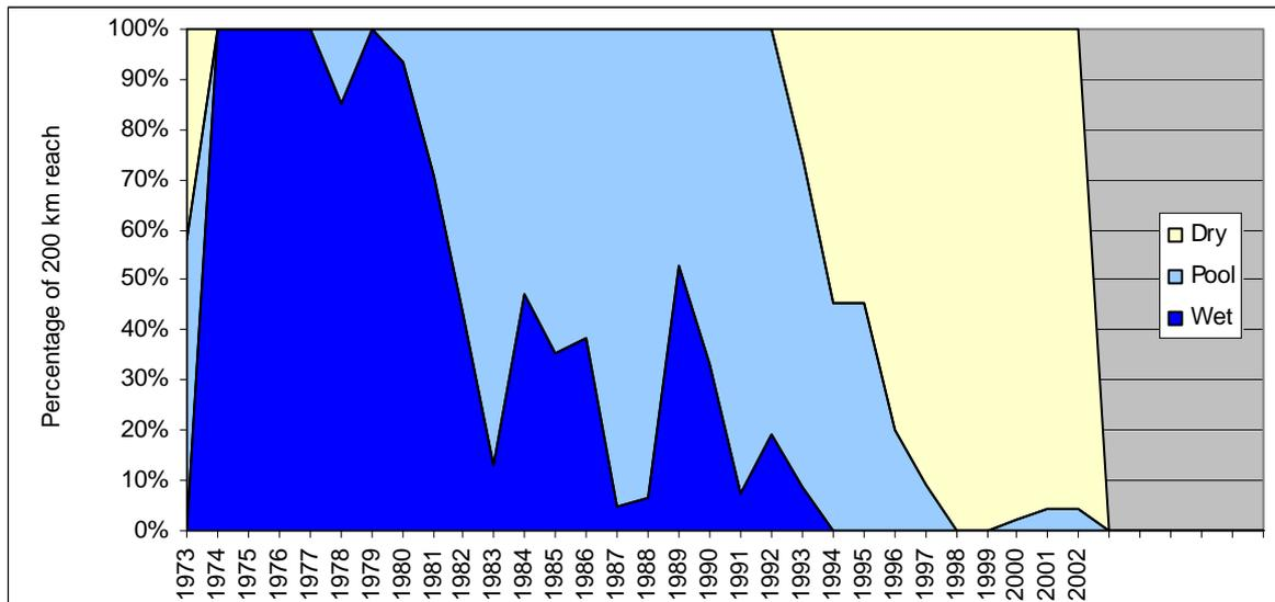
**Figure 5-13 : Percentage of the Boteti River study reach that will be inundated (wet); isolated pools (pool) and dry under the Present day Scenario**
