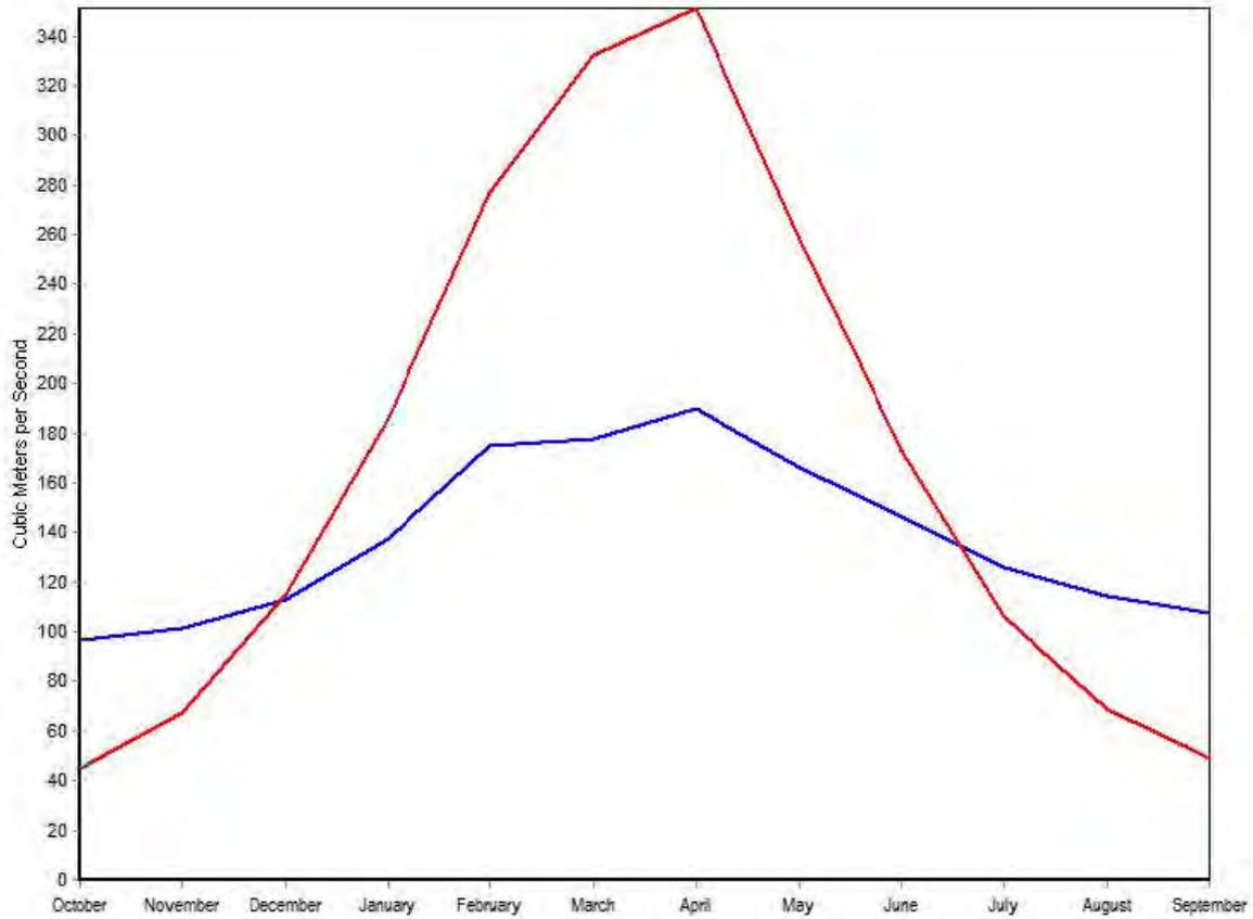
Figure E-4 : Simulated hydrographs of the Cuito River (blue) and Cubango/Kavango River (red)
