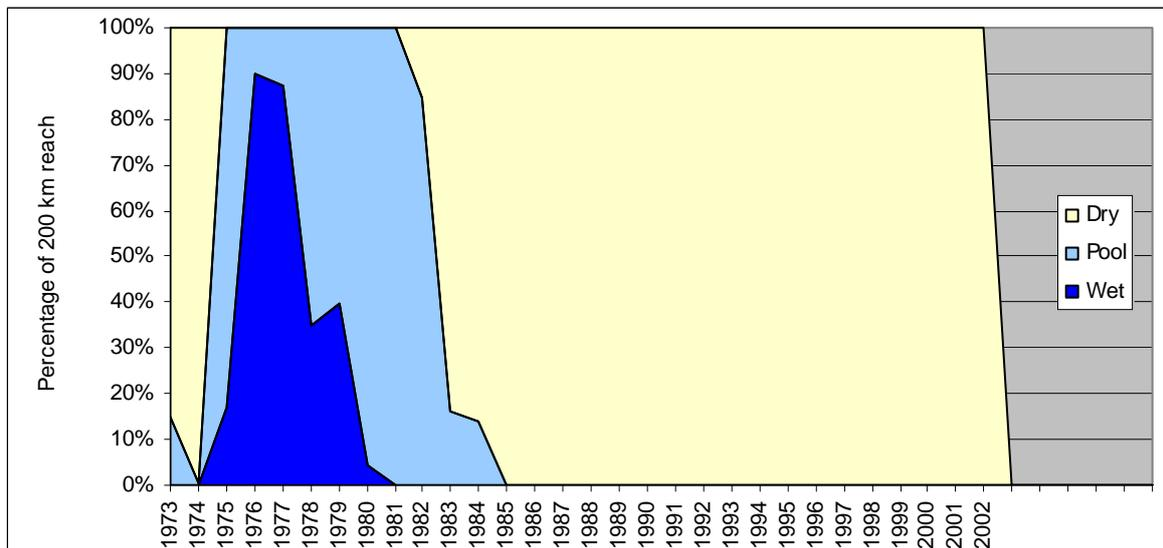
Figure 5-16 : Percentage of the Boteti River study reach that will be inundated (wet); isolated pools (pool) and dry under the High Scenario
