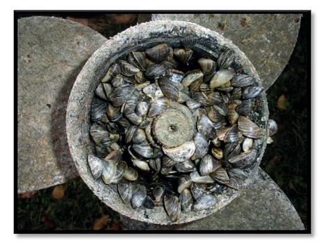
Picture 6: Zebra mussels attached to a boat propeller (Author: T. Britt - Source: Flickr commons).
