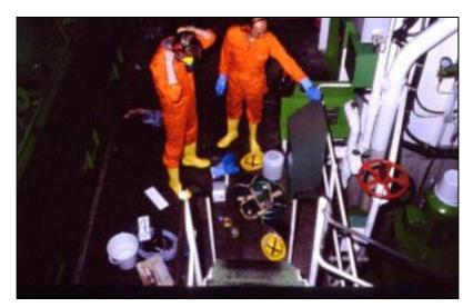
*Figure 6.* Preparation of ballast water sampling in engine room. Safety gear shown (ear protection, aerosol filter, safety rubber boots, gloves, helmet and overall).
