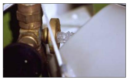
Figure 5.Water sampling at pressure meter of ships ballast pump.
