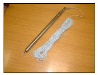
Figure 3. The "Bottom and Sediment Sampler".
