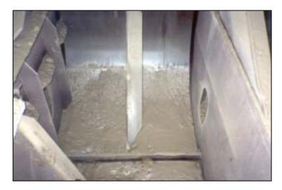
Example of sediment accuumlation in a ballast tank, requiring special sampling techniques (photo: D Oemcke)
