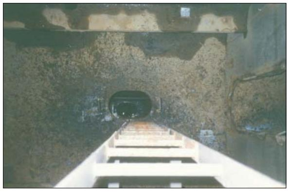
Figure 1b. Complex internal architecture of an empty wing tank.
