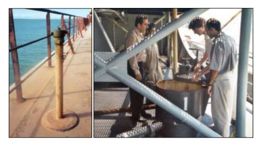
Two points of access for ballast water samplng: Left – ballast tank sounding pipe (photo: D Oemcke); right – ballast tank manhole. Access via the sounding pipe is quicker, but is more restricted and less representative than via the manhole.
