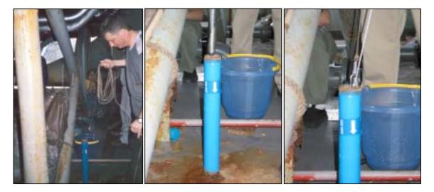
Slovenian ballast water expert Matej David (left) demonstrating deployment of the botton & sediment sampler via a sounding pipe aboard the 'Marajo' (photos: A L Neto)
