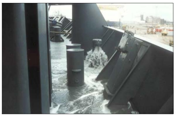
Figure 1e. Ballast tank being overflowed to allow collection of samples.
