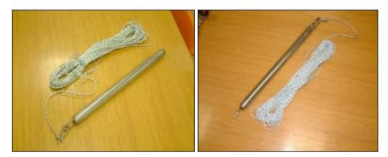
The Slovenian 'Water-Column Sampler' (left) and 'Bottom and Sediment Sampler' (right) suitable for deployment via the ballast tank sounding pipe (photo: M David)
