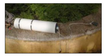
A Van Doorn water sampler capable of collecting several litres of ballast water via the ballast tank manhole (photo: M David)
