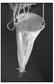
Figure 5. Plankton net (20  $\mu$ m mesh size) for concentrating water sample.
