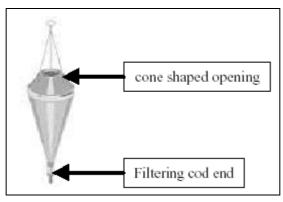
Figure 1. Cone net with filtering cod end.
