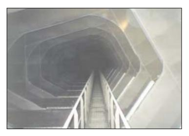
Example of internal ballast tank structure (large bulk carrier), presenting sampling obstacles (photo: D Oemcke)
