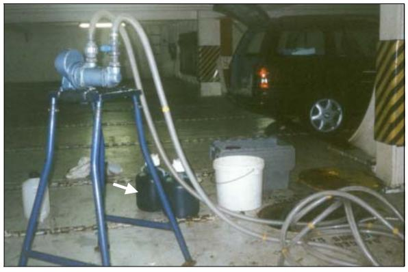
*Figure 1a.* Sampling equipment being used to collect sediment slurry (arrow) via ballast tank hatch from a double bottom tank of a car transporter.
