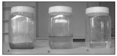
Figure 6. Rusty ballast water (A), oily ballast water (B) and clear ballast water (C).
