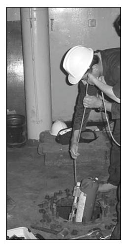
Figure 1. Sampling in the cement ship MARGRANEL by means of the opening of the tank.
