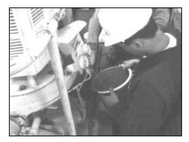
Figure 3. Sampling in the container ship SEA PUMA by means of ballast Pumps.
