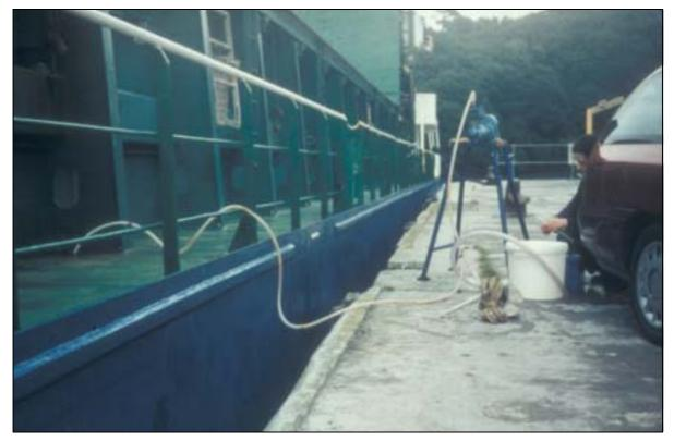
Figure 1c & d. Reinforced hose pushed down a sounding pipe for collection of sediment slurry.
