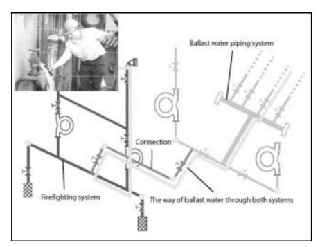
*Figure 4.* The connection of the ballast water and fire-fighting system. The inserted photo shows the ballast water release from the tap on the main deck.
