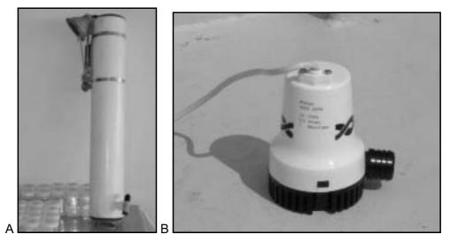
Figure 4. Van-dorn bottle 9 liter capacity (A) and electric pump (B) using for sampling.
