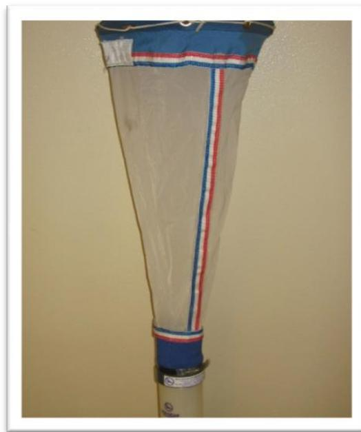
*Figure 17. Plankton Net (35 micrometers) with Attached 1 Liter Cod-End.*
