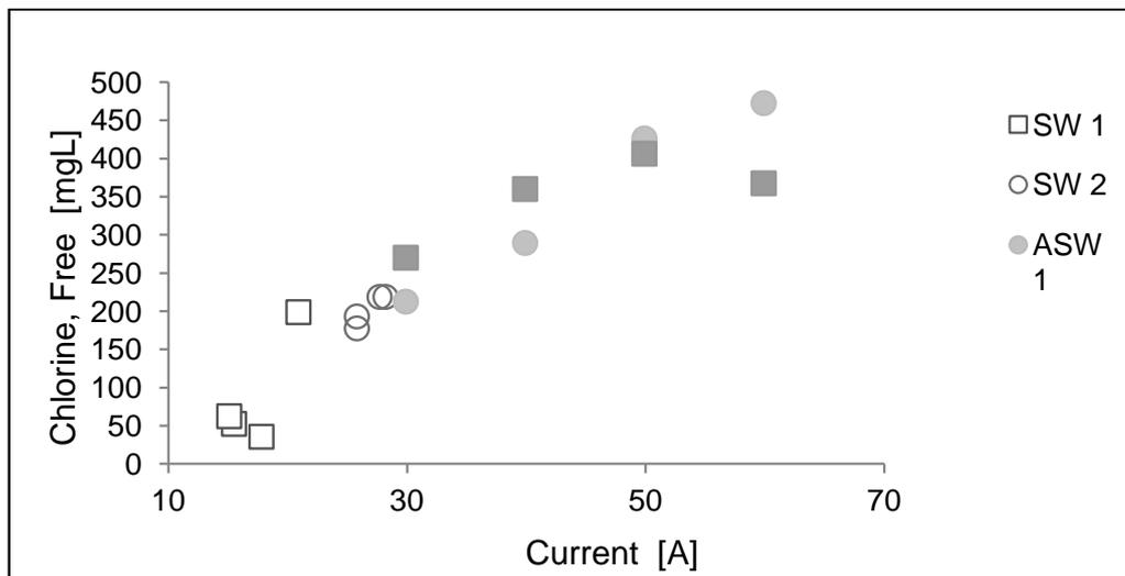
**Figure 7. Effect of substrate on free available chlorine**
