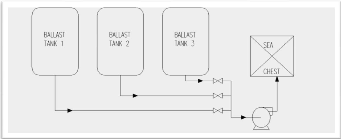
**Figure 4. Schematic of Centralized Manifold Ballast System Design.**
