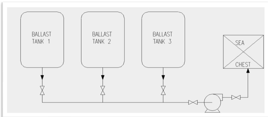
**Figure 3. Schematic of Distributed Manifold Ballast System Design.**
