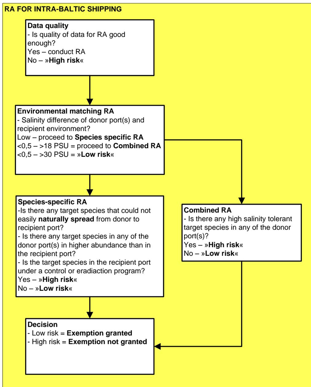
*Figure 1. Risk assessment (RA) methods and principles for granting exemptions from ballast water management in intra-Baltic shipping.*
