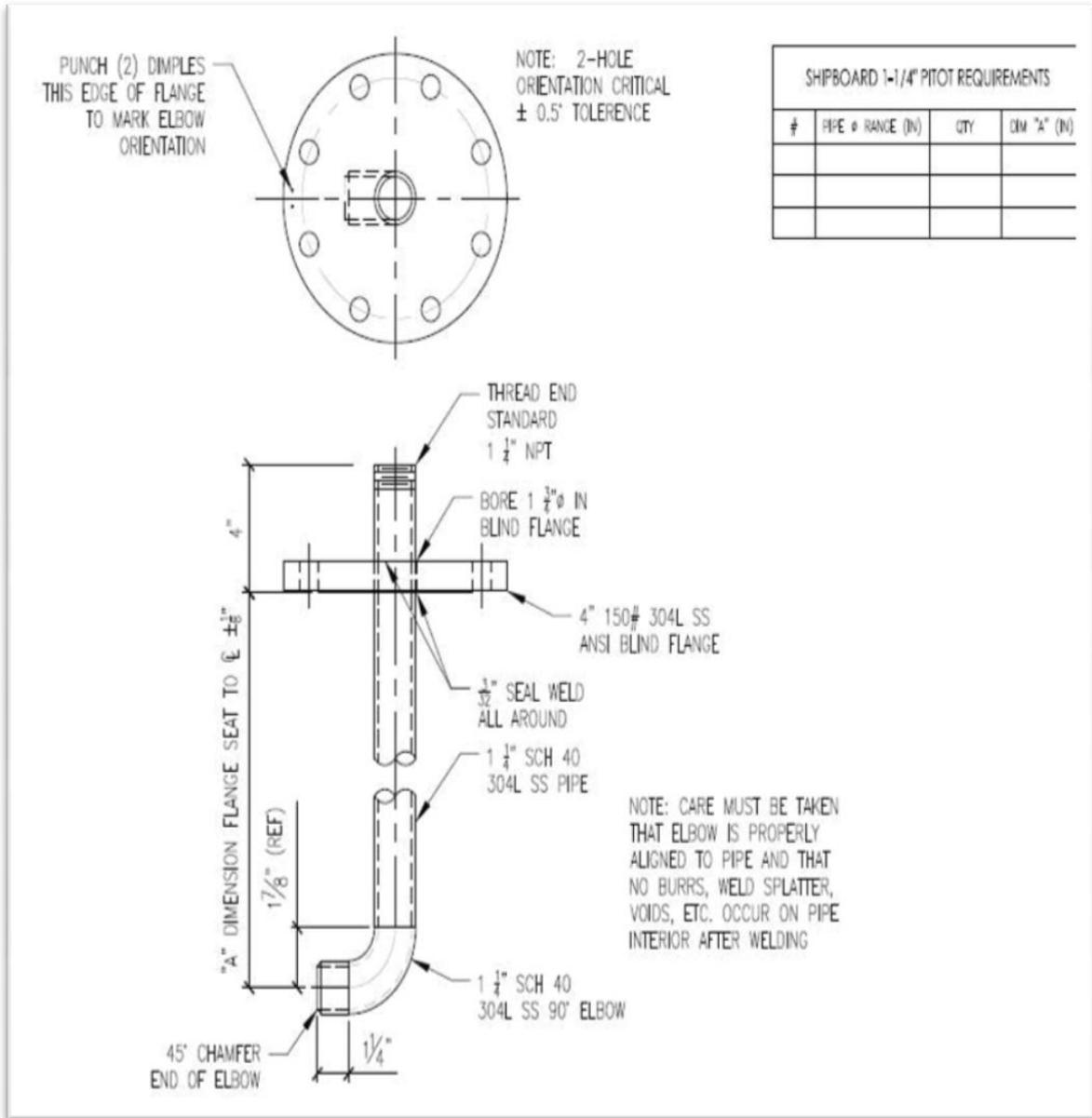
**Figure 2. Diagram of Elbow Pitot for Ballast Discharge Sampling.**
