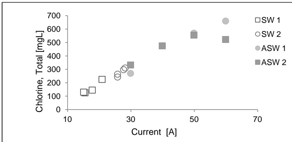
**Figure 6. Effect of substrate on total chlorine**
