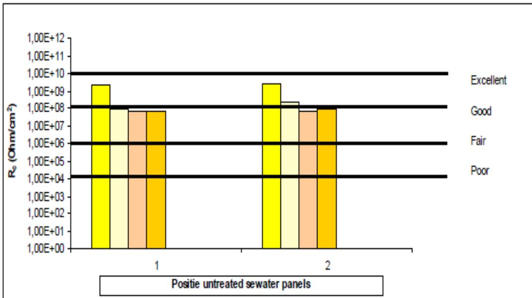
**Figure 7. Development of coating resistance in untreated seawater after 1 day, 30 days, 60 days and 90 days.**
