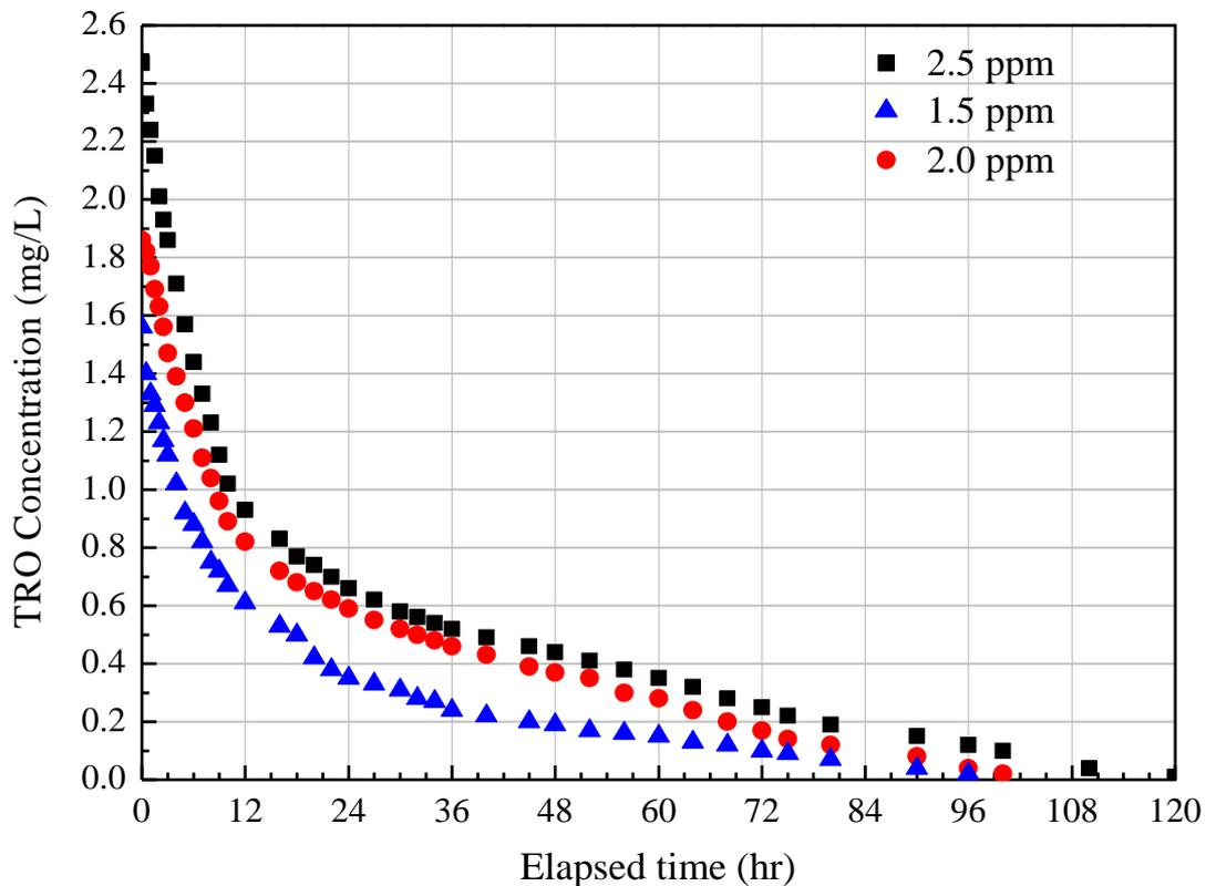
Figure 4. TRO decay over a period of 120h for high salinity (measured as Cl<sub>2</sub>).
