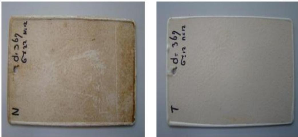
**Figure 4. Intact coated panels in untreated water for 90 days (left) and intact coated steel panels in treated water for 90 days (right).**
