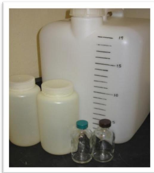
**Figure 18. Sample Collection Containers used for Shipboard Sampling Events.**
