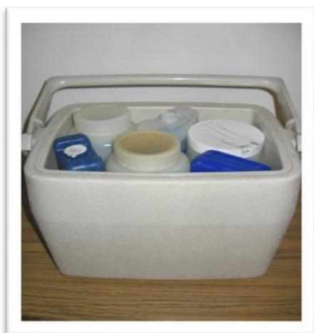
*Figure 19. Small Sample Transport Cooler with Samples and Ice Packs.*
