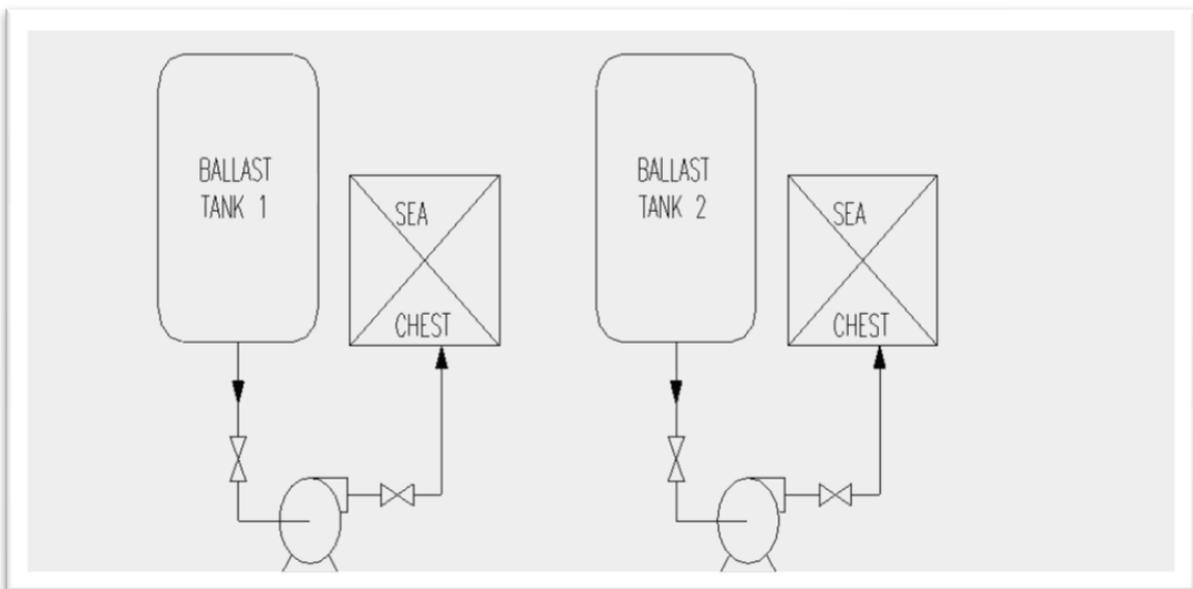
**Figure 5. Schematic of Multiple Independent Ballast System Design.**
