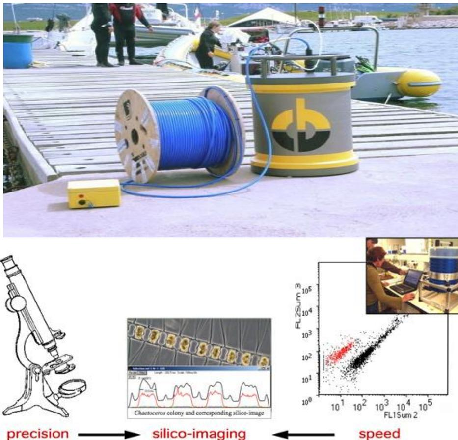
**Figure 3. Buoy equipped for flow cytometry detection [ 5 ].**
