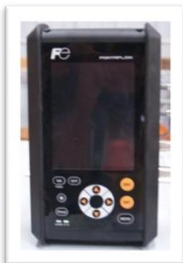
**Figure 8. Ultrasonic Flow Meter.**
