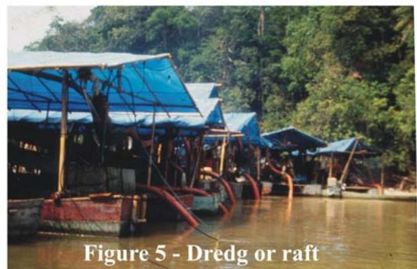
The motor engines with larger potencies move a centrifugal pump adapted to two hoses with diameter from 4 to 6 inches. In one of the hose, whose extremity is inside water, has the *abacaxi* scrapper (garimpeira denomination to define metallic cylinder to make the suction of gravel or mineralized level). The *abacaxi* makes suction of the gravel or mineralized level from drainage's bed, underwater, that is
