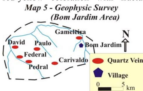
The deposit typology is composed by three auriferous quartz veins, with directions to the N80°E and N50°E. They have in surface an extension of approximately 400 m length and with thickness between 0.40 and 1.50 m. The
