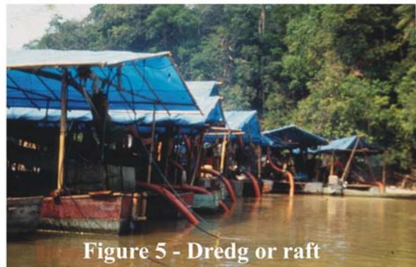
The motor engines with larger potencies move a centrifugal pump adapted to two hoses with diameter from 4 to 6 inches. In one of the hose, whoses extremity is inside water, has the *abacaxi* scrapper (garimpeira denomination to define metallic cylinder to make the suction of gravel or mineralized level). The *abacaxi* makes suction of the gravel or mineralized level from drainage's bed, underwater, that is
