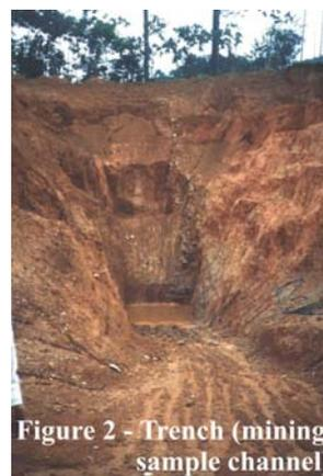
Figure 2 - Trench (mining sample channel)
