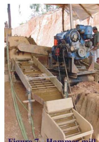
Figure 7 - Hammer mill
