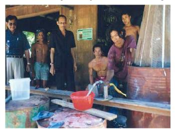
Photo 2 – Miners in Guha using the home-made retort
