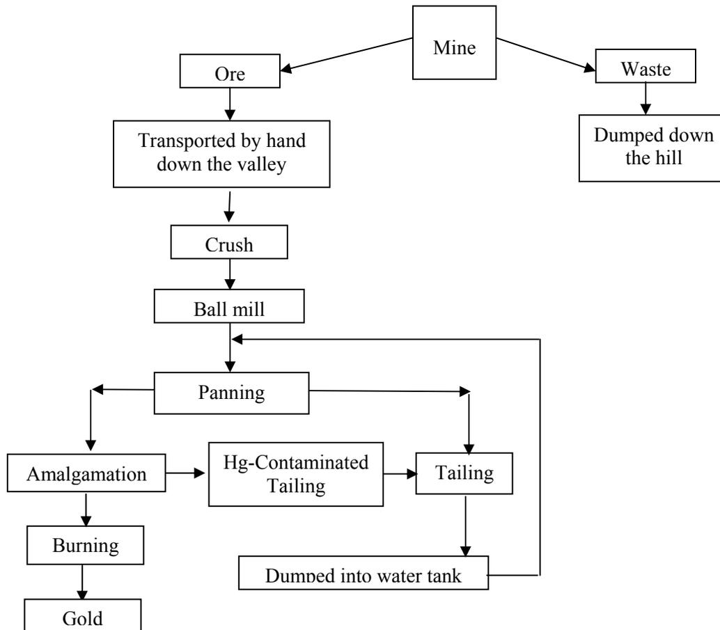
Fig. 1 – Flowchart of Mining and Milling Operations in Munhena
