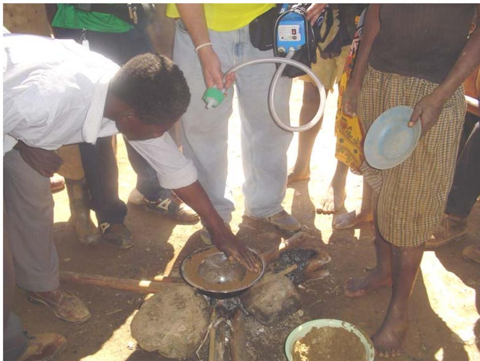
*Measuring the reduction of Hg emission when using the retorts*
