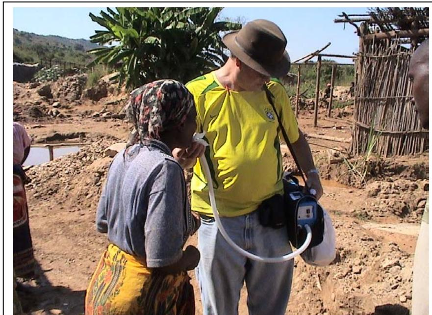
*Testing mercury levels in breath*
