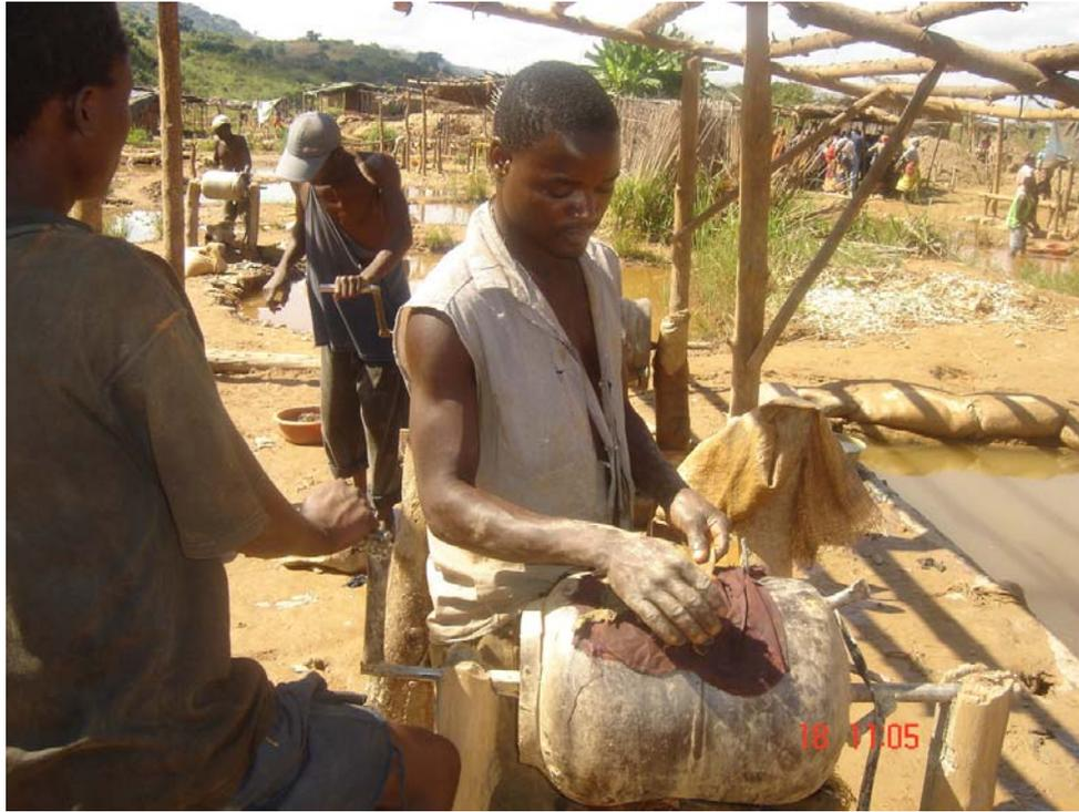
*Propane tanks transformed into ball mills*
