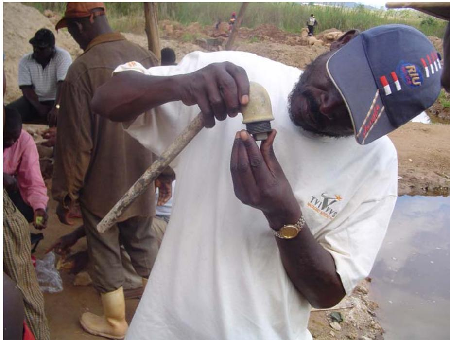
*Miner using the water-pipe retort*
