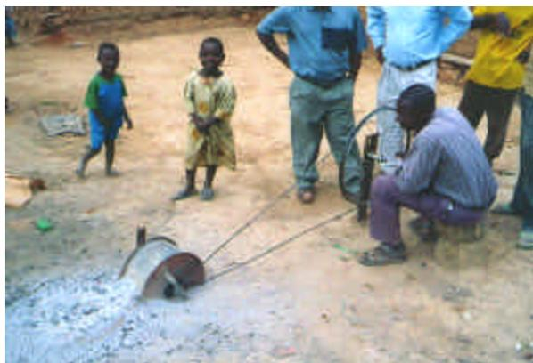
*Fig. 1 – Home-made air blower to forge steel tools: this can be used for more efficient retorting*
