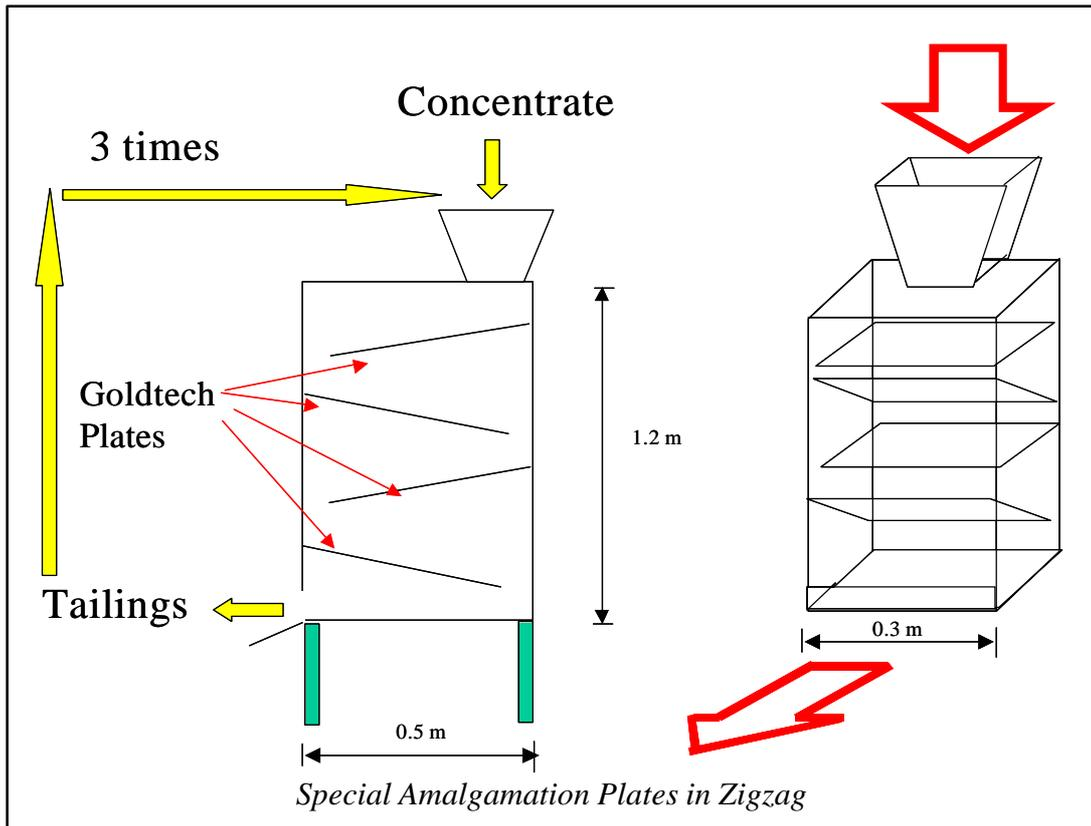
**Table 3.10 – Technical Data of a Box with Special Amalgamation Plates in Zigzag**
