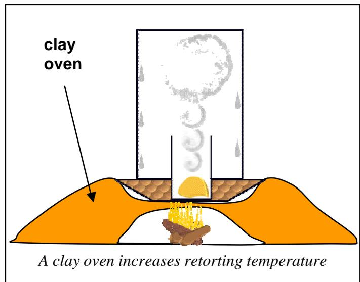
Using a glazed-steel (enameled) bowl as crucible, yellow gold is obtained, increasing the acceptability of miners to the retorting process. The firing structure can also be built in clay as used in Western Africa for cooking. This process increases the temperature of the bonfire and concentrates the flames under the bowl.
