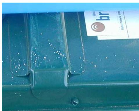
B: Mercury droplets on the metal box
