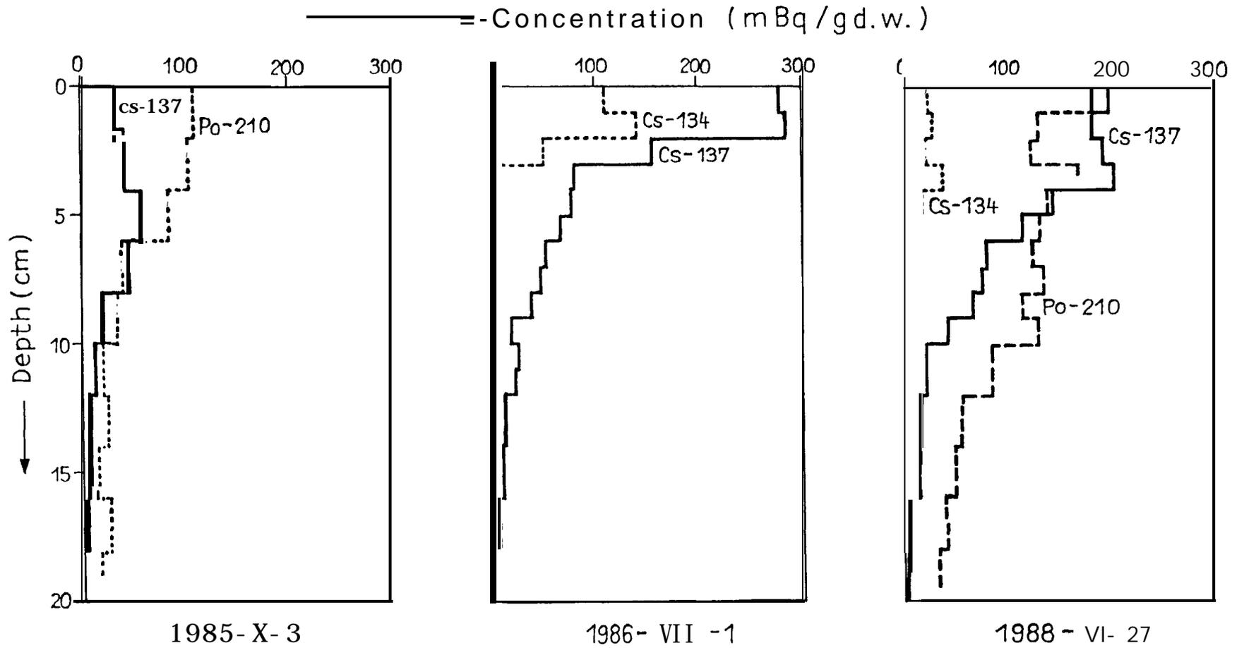
Figure 7: Depth penetration of radiocesium along a sediment core (Greifswald Bodden)
