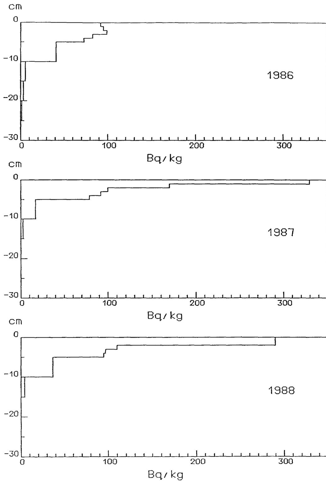
Fig. 6. Vertical distribution of cesium-137 ( $\text{Bq kg}^{-1}$  dry wt.) in sediment samples taken at the Teili-1 station in 1986-1988.
