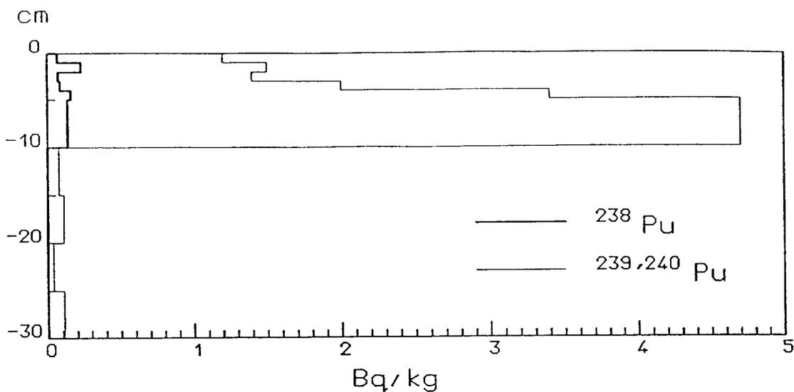
Fig. 7. Vertical distribution of plutonium-238 and plutonium-239,240 ( $\text{Bq kg}^{-1}$  dry wt.) in sediment samples taken at the Teili-1 station in 1988.
