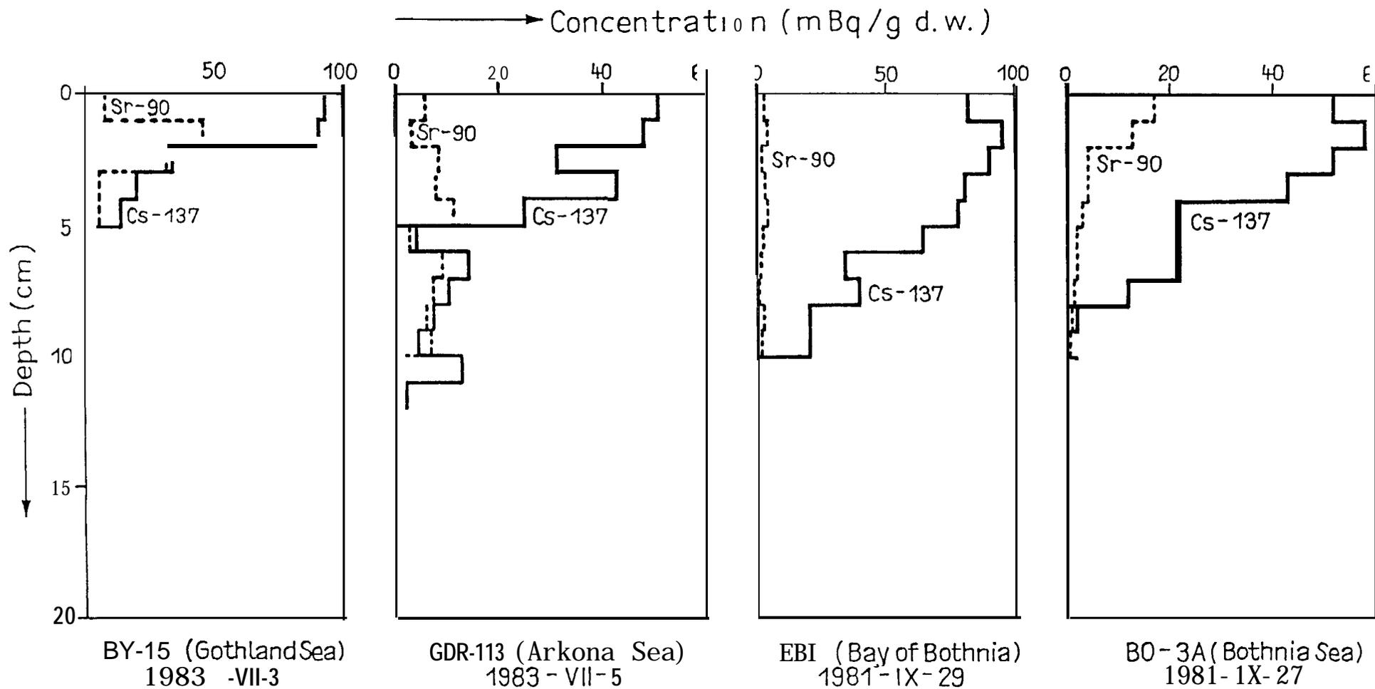
Figure 1: Distribution of Sr-90 and Cs-137 along sediment cores from different parts of the Baltic Sea
