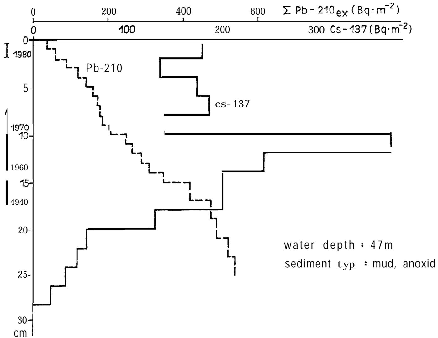
Figure 2 :Radionuclide distribution along a sediment core, Arkona basin , 1984
