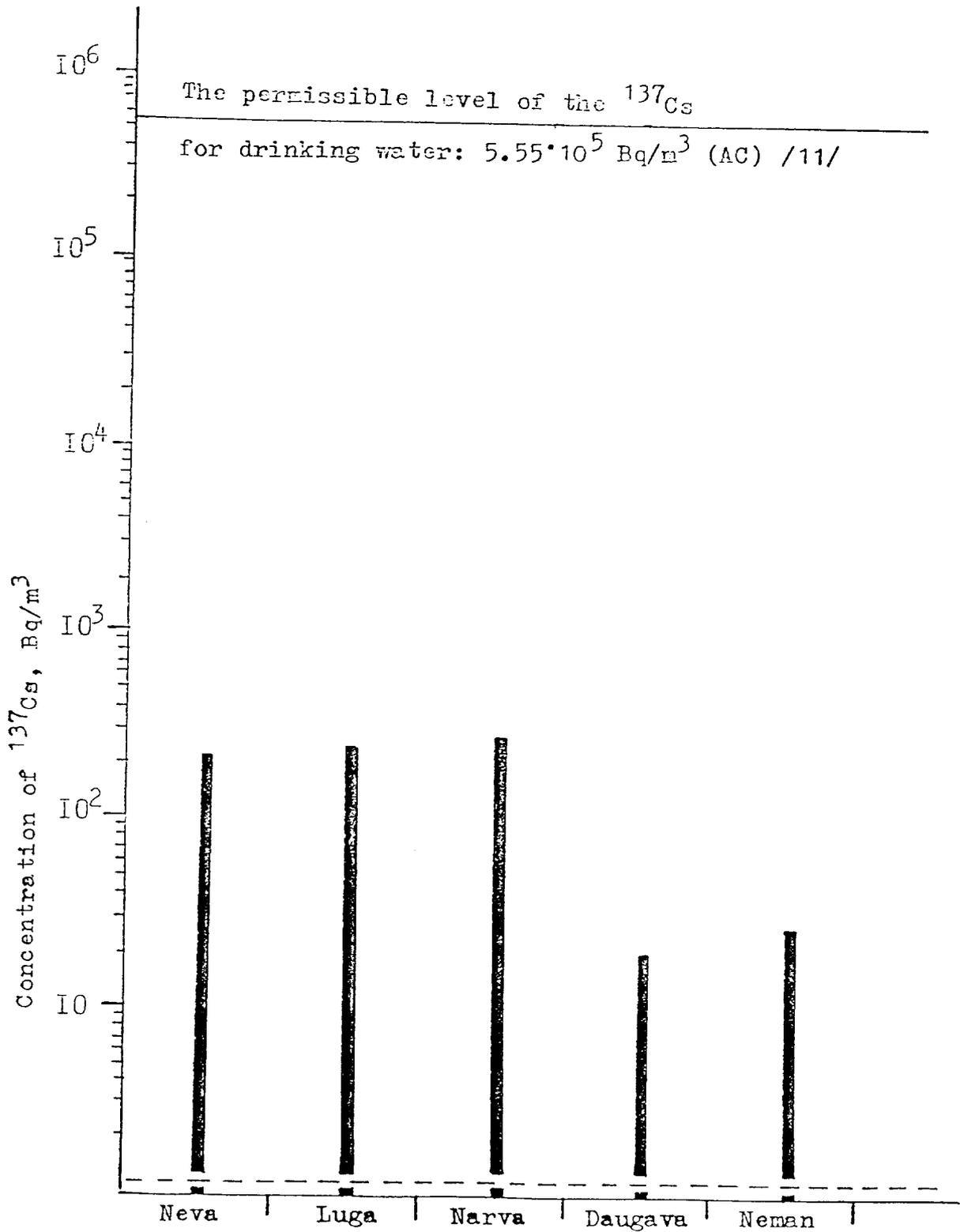
Fig. 2. Values of  $^{137}\text{Cs}$  content ( $\text{Bq/m}^3$ ) in the water of the rivers in May-July 1986 relative to the background level and the AC (acceptable concentration).
