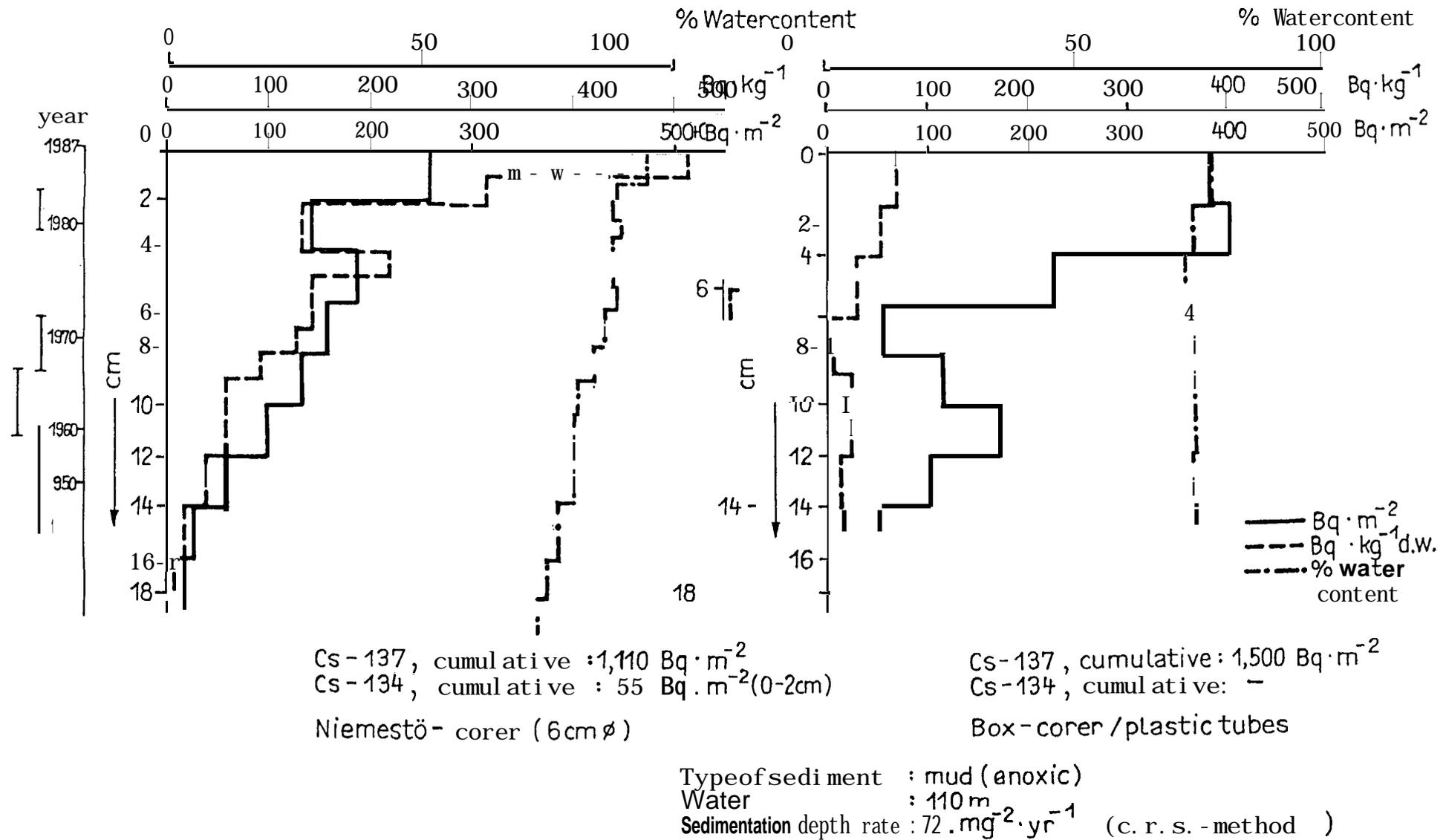
Figure 8: Distribution of Cs-137 along sediment core profiles in dependence on the type of sediment sampler, Stat. 25 (Bay of Gdansk), VIII/ 1987
