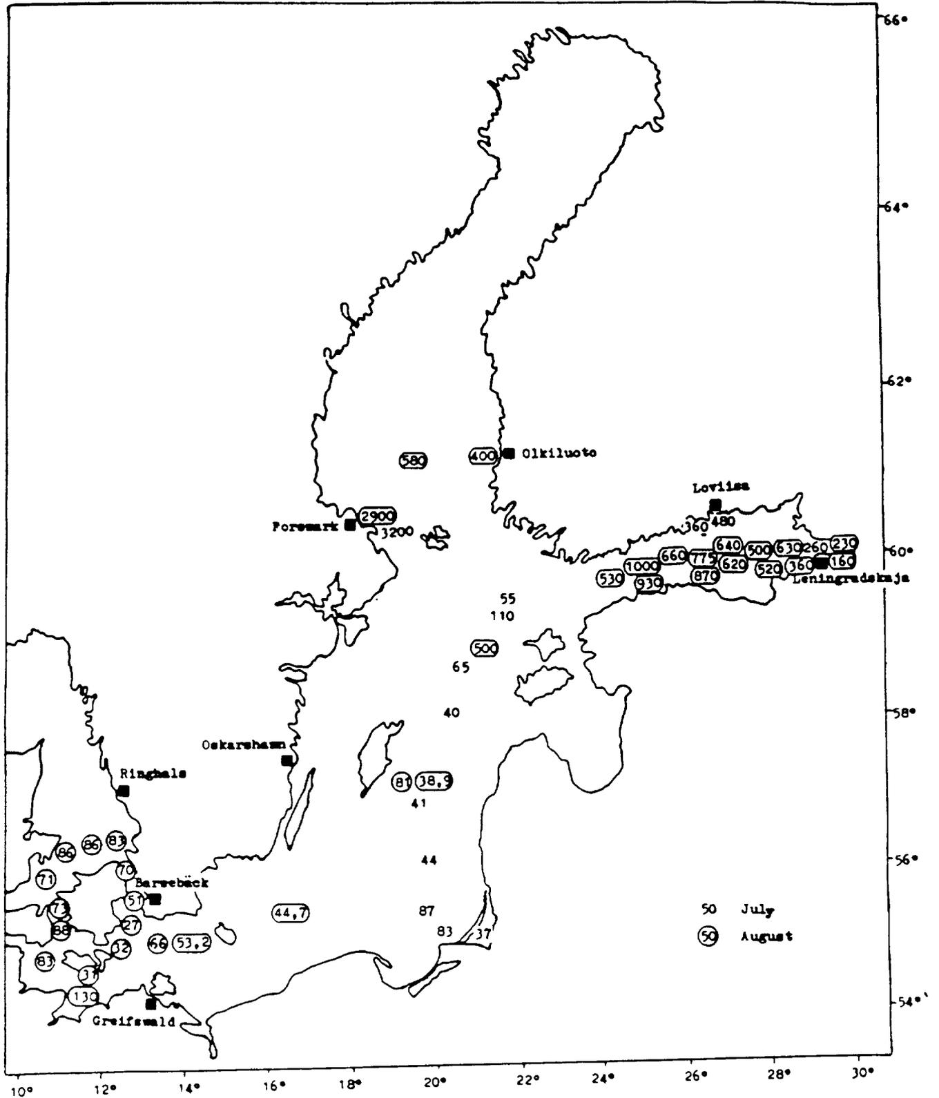
Fig. 2.  $^{137}\text{Cs}$  activity concentration, Bq/m<sup>3</sup>, in the surface water of the Baltic Sea in July-August 1986.
