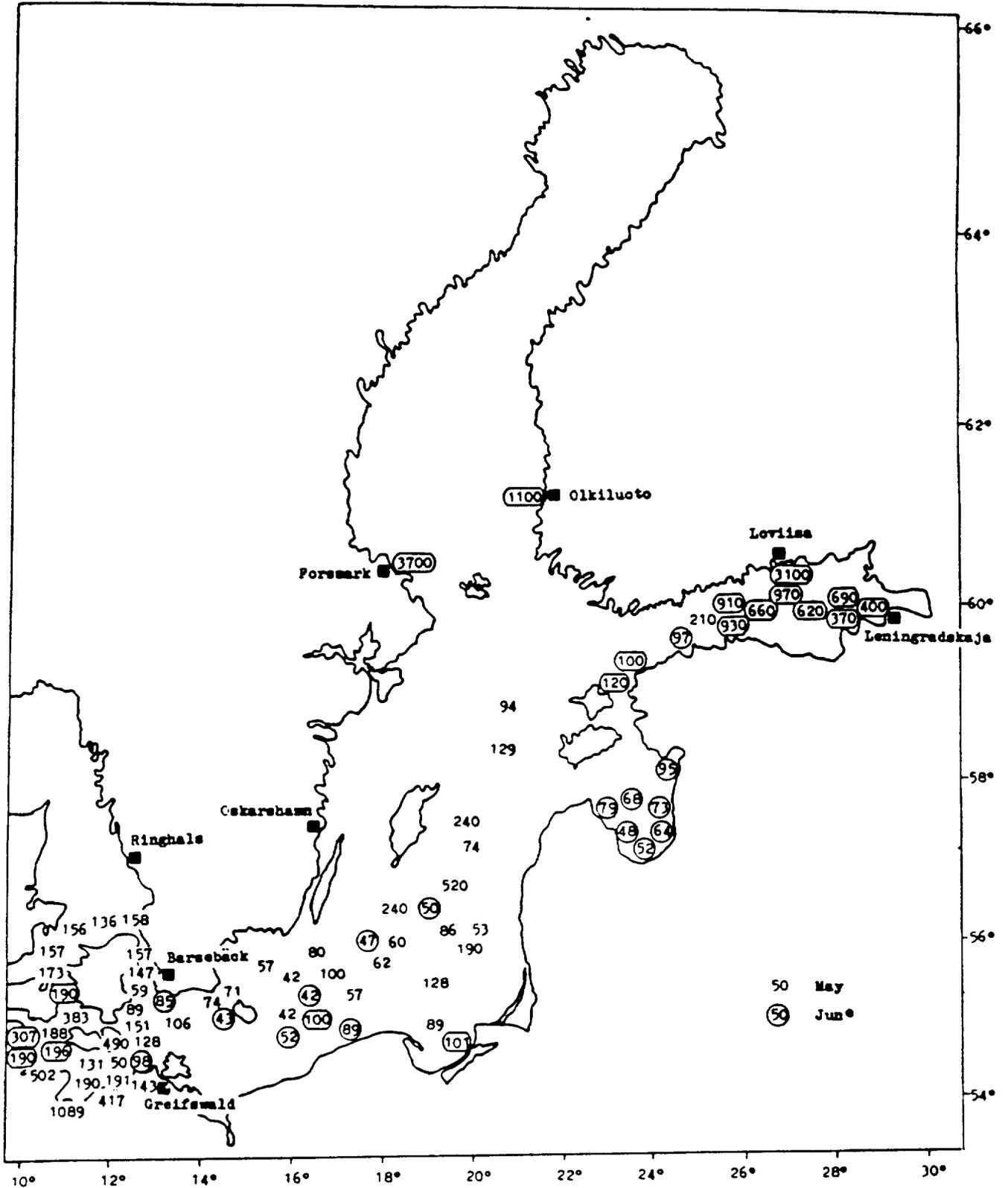
Fig. 1.  $^{137}\text{Cs}$  activity concentration,  $\text{Bq/m}^3$ , in the surface water of the Baltic Sea in May-June 1986.
