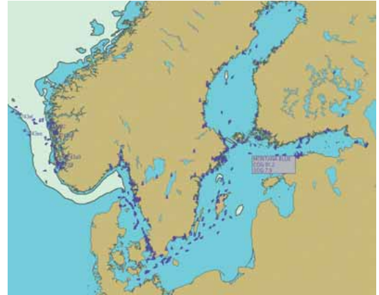
Images based on AIS information show the current positions of ships in the Baltic Sea. This map only includes ships in waters presently covered by land-based AIS stations.
