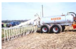
Drag hose tractor: precise fertilization, around 41% lower NH 3 emissions
