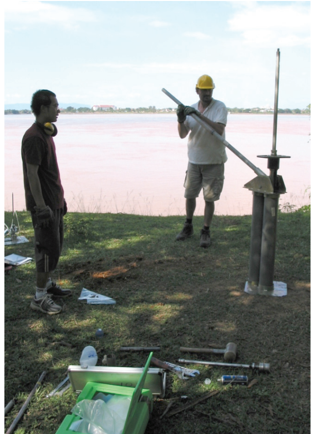
Core samples of soils are used as models of riverside stability.
