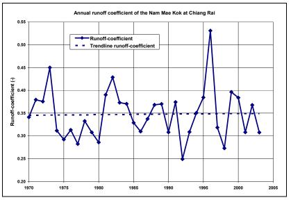
Figure 3.18 Runoff-coefficient of the Nam Mae Kok at Chiang Rai
