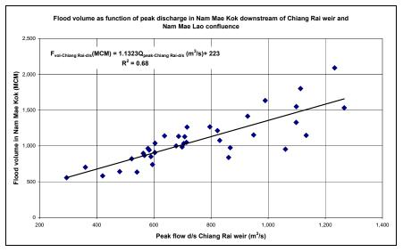
Figure 4.23 Flood volume versus peak flow in Nam Mae Kok at Lao confluence
