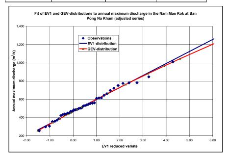
Figure 4.2 Fit of EV1 and GEV-distributions to annual maximum discharge in Nam Mae Kok at Ban Pong Na Kham (adjusted series), Period 1967-2007
