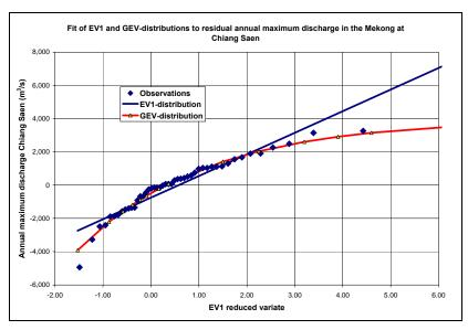
Figure 4.29 EV1 and GEV fit to residual annual maximum discharge in the Mekong at Chiang Saen
