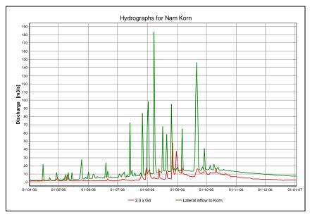
Figure 4.6 Upstream and lateral inflow to hydraulic model of Nam Korn, year 2006
