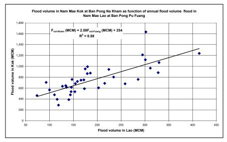
Figure 4.14 Flow volume in Nam Mae Kok at Ban Pong Na Kham during occurrence of peak flow in Nam Mae Lao
