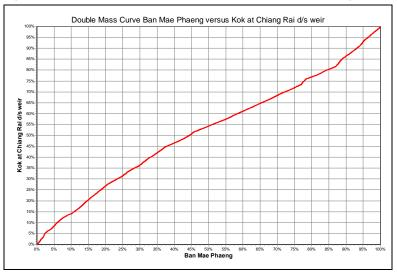
Figure 4.18 Double mass curve of discharge in Nam Mae Kok at Ban Mae Phaeng and at Lao confluence for years 1994-2007
