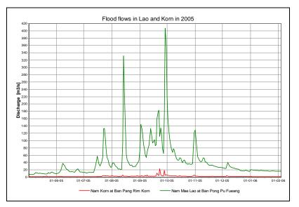
Figure 3.9 Floods of 2005 in Nam Mae Lao at Ban Pong Pu Fuang and Nam Korn at G4
