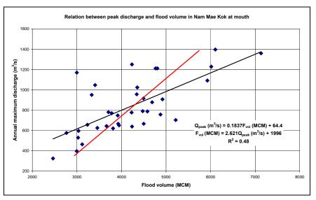
Figure 4.32 Relation between peak discharge and flood volume in Nam Mae Kok at mouth
