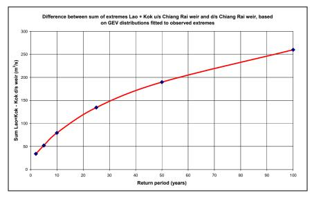
Figure 4.22 Reduction of combined peak discharge d/s Chiang Rai relative to sum of upstream Kok and Lao peaks as a function of return period
