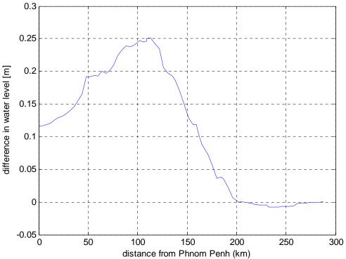
Figure 5.25 Increase in water level in the **Mekong** river downstream of Phnom Penh as a result of scenario **Cam0VNa**.
