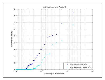
Figure 5.32 Frequency distribution of the total volume above a threshold of 30,000 m<sup>3</sup>/s in the Mekong downstream of Phnom Penh until August 1, depending on the available flow capacity of the diversion channel.
