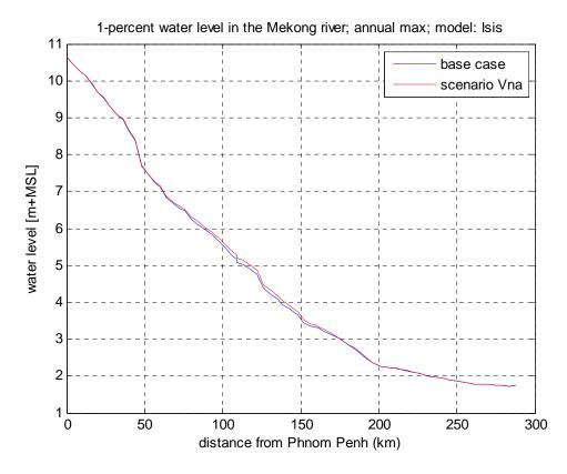
Figure 5.18 Water levels in the **Mekong** river downstream of Phnom Penh; comparison between the base case and scenario **VNa**.
