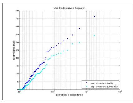
Figure 5.33 Frequency distribution of the total volume above a threshold of 30,000 m<sup>3</sup>/s in the Mekong downstream of Phnom Penh until August 21, depending on the available flow capacity of the diversion channel.
