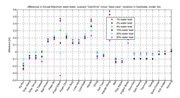
Figure 5.22 Change in the p-percent annual maximum water level (p=1, 2, 4, 10, 20 and 50) for 25 locations in **Cambodia**; comparison of scenario **Cam0VNa** with the base case. Positive values indicate an increase in water level.
