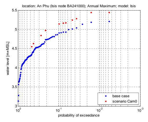
Figure 5.7 Exceedance frequencies of annual maximum water levels of 97 in the base case (blue dots) compared to water levels in 11 selected years.
