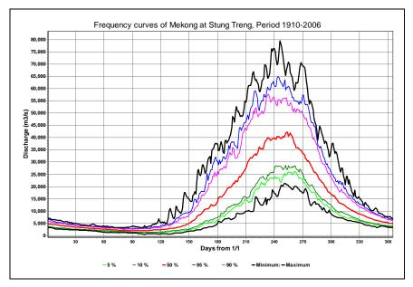
Figure 4.2 Frequency curves of the Mekong discharge at Stung Treng, Period 1910-2006
