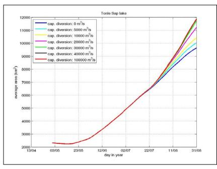
Figure 5.30 Mean wet surface area of the lake for different values of the flow capacity of the diversion.
