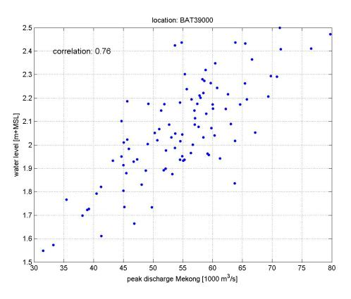
Figure 5.5 Annual peak discharges (1000 m<sup>3</sup>/s) in the Mekong river at Stung Treng versus annual maximum water level at model node BAT39000.
