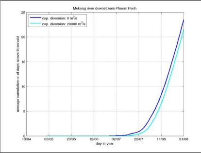
Figure 5.31 Average cumulative number of days (up to the date shown on the horizontal axis) in the simulated period 1910-2006 during which the flow downstream of Phnom Penh exceeded 30,000 m<sup>3</sup>/s; depending on the available flow capacity of the diversion channel.
