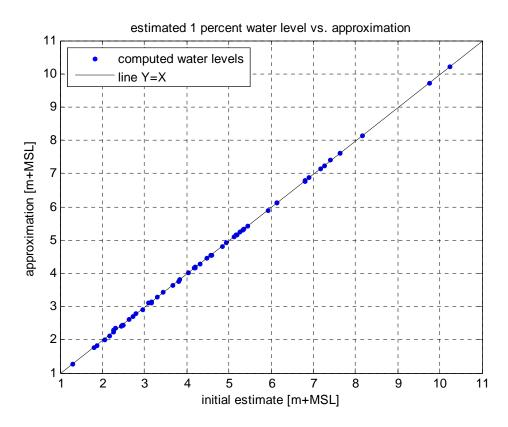
Figure 5.9 Comparison of the estimated 1%-water level (i.e. the 100 year water level) based on 97 simulated years (horizontal axis) and the approximated estimate based on 11 simulated years (vertical axis). The comparison is made for the 59 selected locations.
