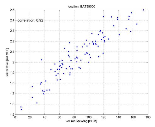
Figure 5.4 Annual flow volumes (BCM) in the Mekong river at Stung Treng above a threshold discharge of 25,000 m<sup>3</sup>/s versus annual maximum water level at model node BAT39000.
