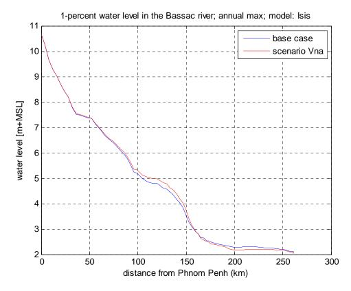
Figure 5.20 Water levels in the **Bassac** river downstream of Phnom Penh; comparison between the base case and scenario **VNa**.
