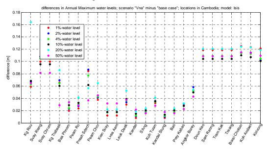
Figure 5.16 Change in the p-percent annual maximum water level (p=1, 2, 4, 10, 20 and 50) for 25 locations in **Cambodia**; comparison of scenario **VNa** with the base case. Positive values indicate an increase in water level.
