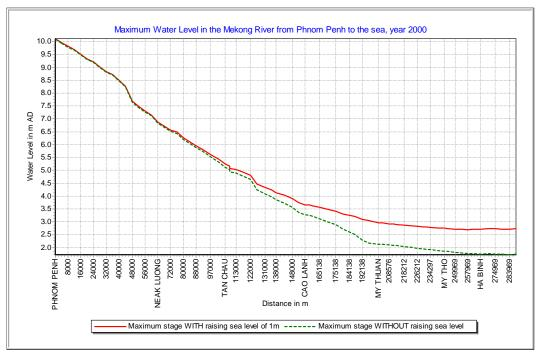
Figure 5.35 Net effect of 1 m sea level rise on the maximum water levels in Bassac, conditions of year 2000
