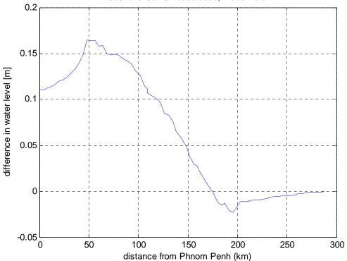
Figure 5.13 Increase in water level in the **Mekong** river downstream of Phnom Penh as a result of scenario **Cam0** (differences between the two cases of Figure 5.12).
