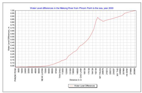
Figure 5.37 Net effect of 1 m sea level rise on the maximum water level in Mekong, conditions of year 2000
