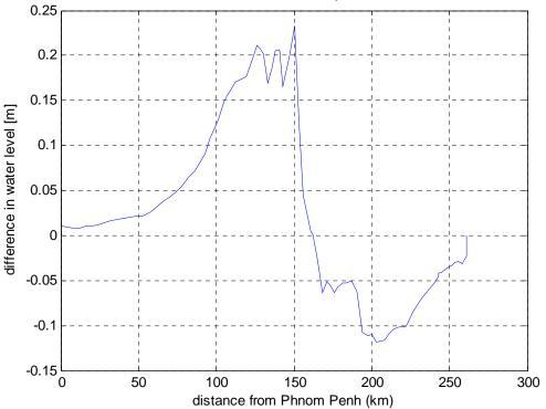
Figure 5.21 Increase in water level in the **Bassac** river downstream of Phnom Penh as a result of scenario **VNa**.
