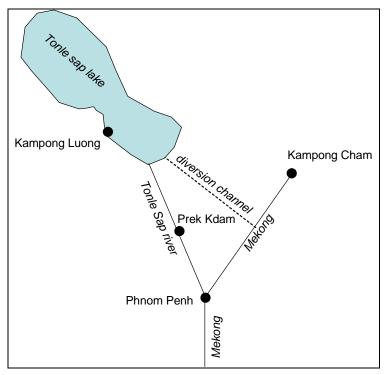
Figure 5.28 Structure of water balance model of Mekong and Tonle Sap
