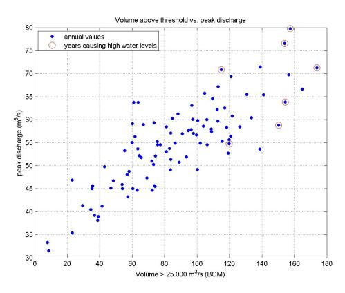
Figure 5.3 Volume of flow above the threshold of 25.000 m<sup>3</sup>/s versus peak discharge
