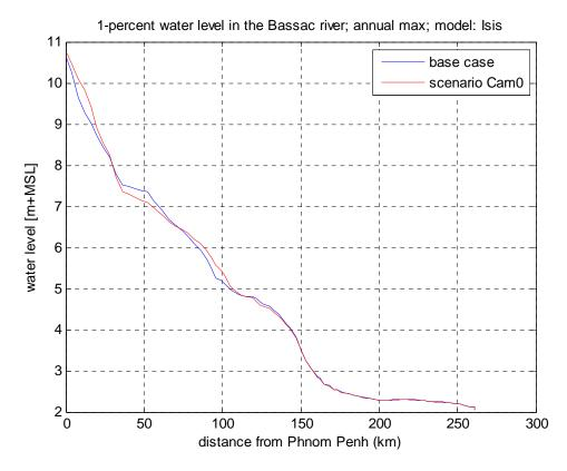
Figure 5.14 Water levels in the **Bassac** river downstream of Phnom Penh; comparison between the base case and scenario **Cam0**.
