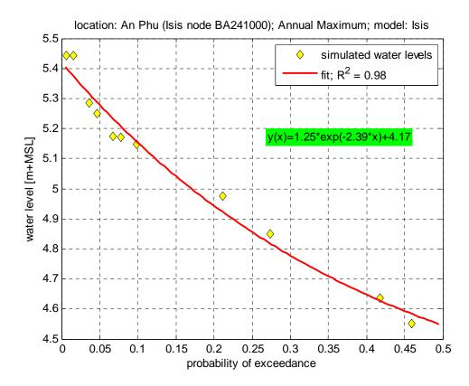
Figure 5.6 Fitted function of probability of exceedance for water levels for location An Phu; Base case.
