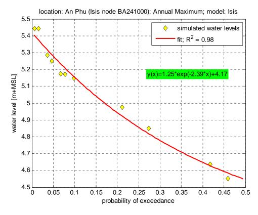
Figure 5.8 Fitted function of probability of exceedance for water levels for location An Phu; scenario Cam0
