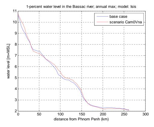
Figure 5.26 Water levels in the **Bassac** river downstream of Phnom Penh; comparison between the base case and scenario **Cam0VNa**.
