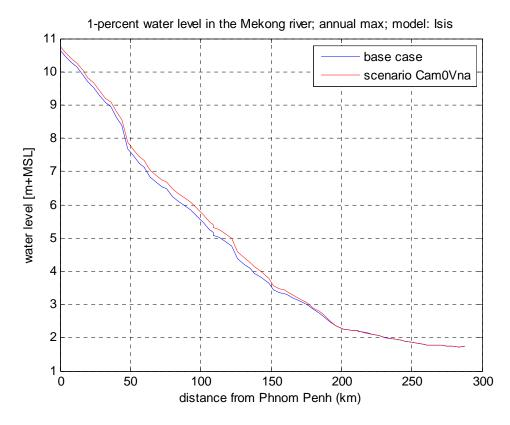
Figure 5.24 Water levels in the **Mekong** river downstream of Phnom Penh; comparison between the base case and scenario **Cam0VNa**.
