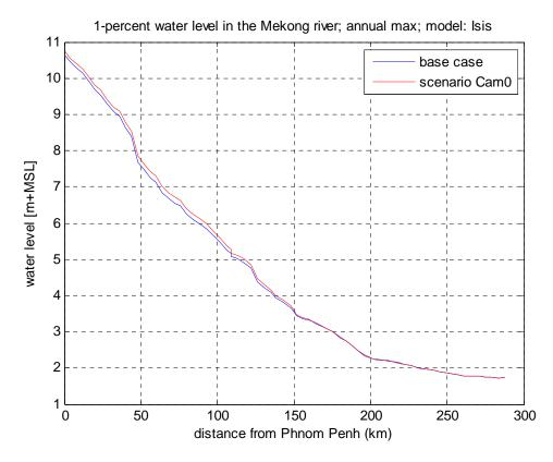
Figure 5.12 Water levels in the **Mekong** river downstream of Phnom Penh; comparison between the base case and scenario **Cam0**.
