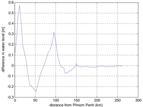
Figure 5.15 Increase in water level in the **Bassac** river downstream of Phnom Penh as a result of scenario **Cam0** (differences between the two cases of Figure 5.14).
