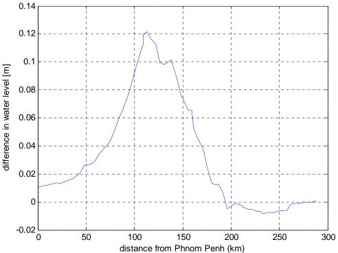
Figure 5.19 Increase in water level in the **Mekong** river downstream of Phnom Penh as a result of scenario **VNa**.
