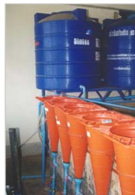
Figure 6. Funnel-type incubator
