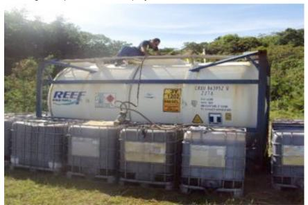
Figure 8: Waste Oil transfer for transport
