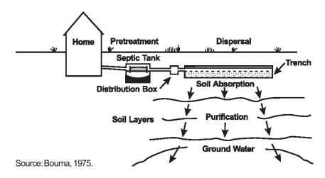
Figure 6: Soil absorption trench. Source (Bouma, 1975)
