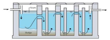
Figure 4: Anaerobic Baffle Reactor. Source (Morrell & Diener, 2006)
