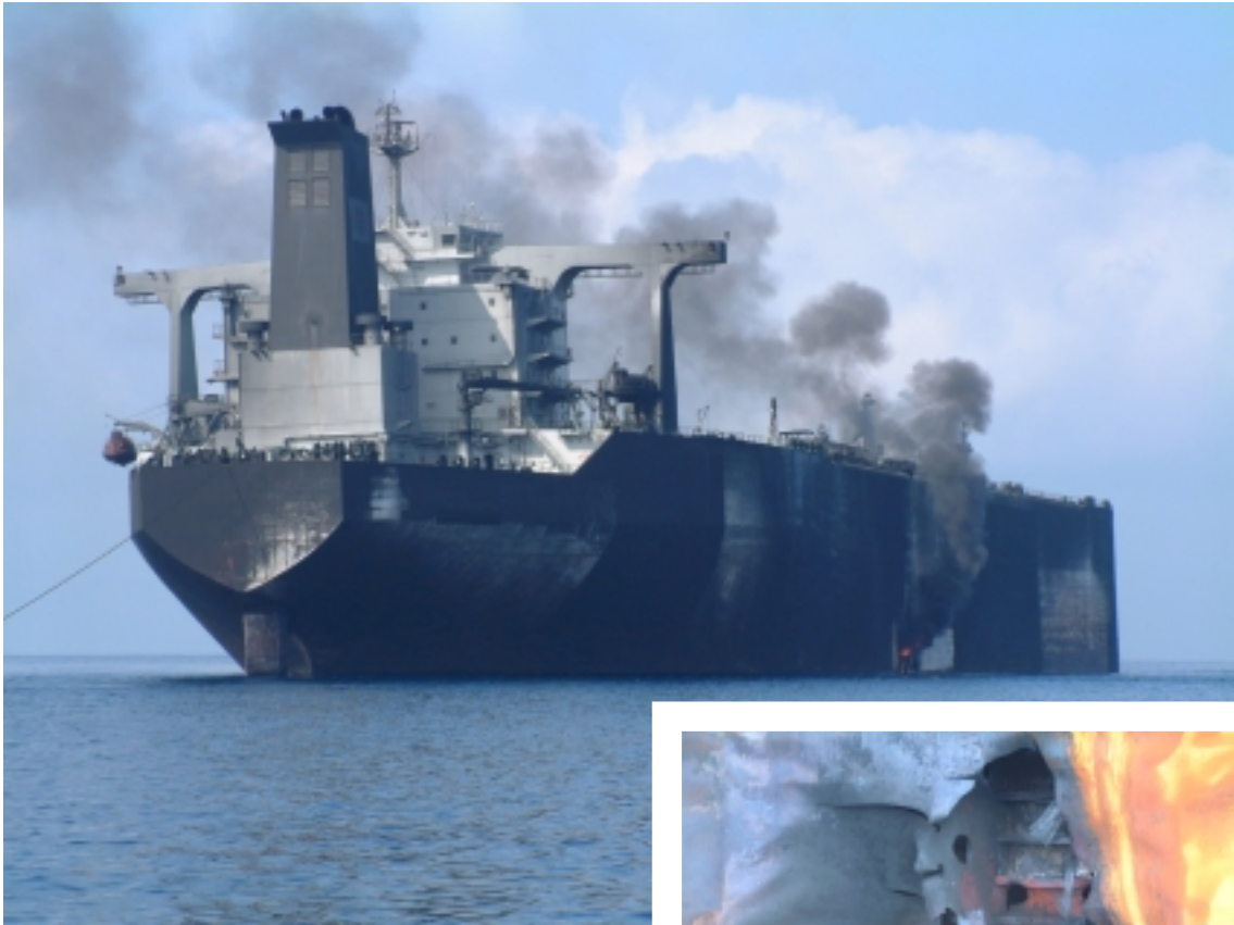
MV Limburg burning off the southern coast of Yemen, October 2002; the hole opens through the double skin of the tanker (NEXEN Petroleum, Capt. R. Facey)
