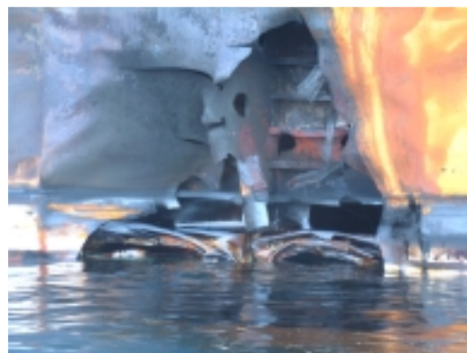
MV Limburg burning off the southern coast of Yemen, October 2002; the hole opens through the double skin of the tanker (NEXEN Petroleum, Capt. R. Facey)
