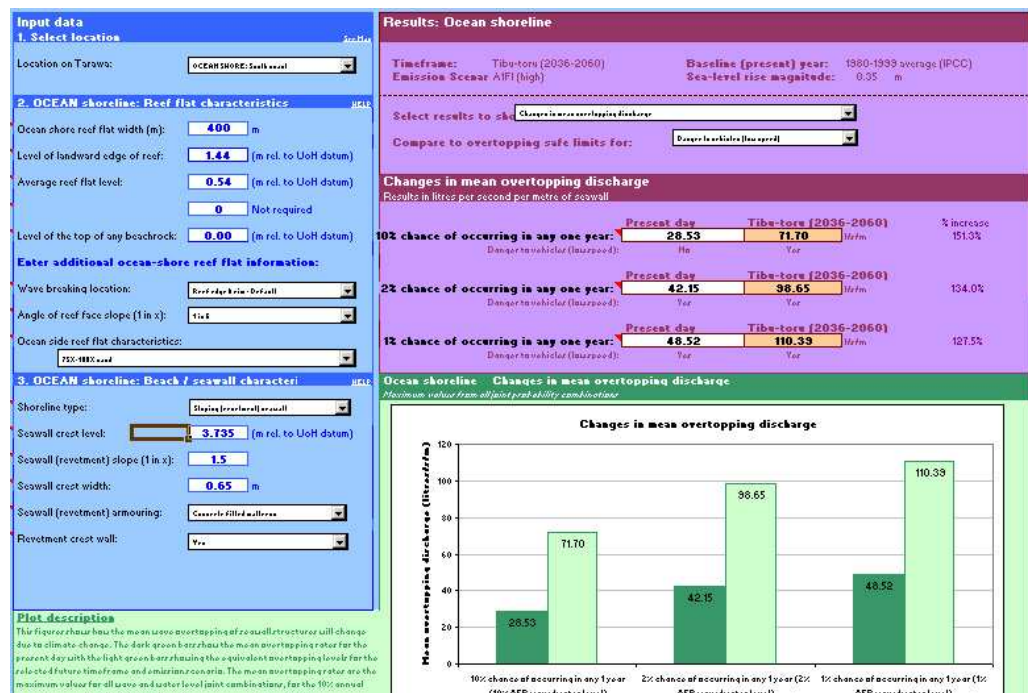
Figure 5: Example of the calculator tool developed to assess climate change and sea-level rise impacts on coastal inundation drivers as part of the Kiribati Adaptation Project.
