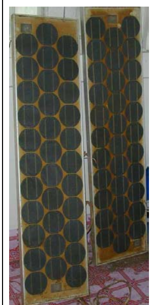
Figure 6-1 - Corroded BP Solar Panels from 1985 Ha'apai projects
