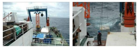
Figure 103. Deployment of ROV KIEL 6000 from the stern gantry of RRS James Cook. ROV still on deck (left) and in the water released from its latch (right). Photos: Aurélie Spadone,/ IUCN
