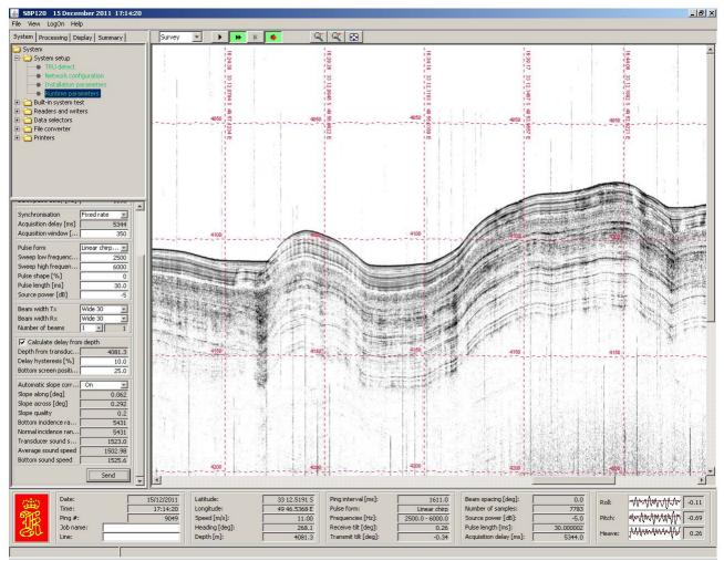
Figure 75. SBP Penetration off the sea mounts and during transit were greatly improved.
