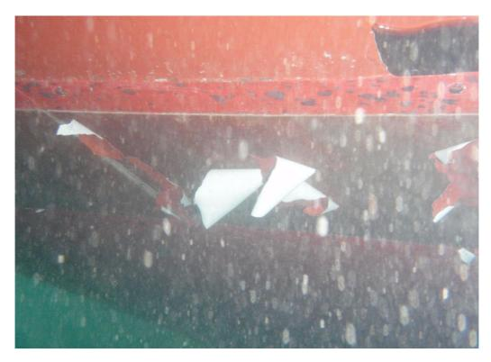
Figure 70. Paint peeling on EM120 transducers.
