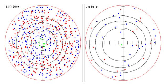
Figure 27. Single target detections of the 120 kHz transducer (left) and the 70 kHz transducer (right) during calibration of the EK60 echosounders on the RRS James Cook. This comparative example (the remaining three transducers were similar to the 120 kHz) shows there are significantly fewer single target detections on the 70 kHz than the other transducers.
