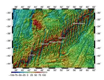
Figure 21. Regional free air anomalies derived from satellite altimetry. N-S fracture zones marked by a gravity low are N-S illustrating the highly oblique spreading direction. Seamounts along the walls of the median valley exhibit gravity highs due to the mass excess.
