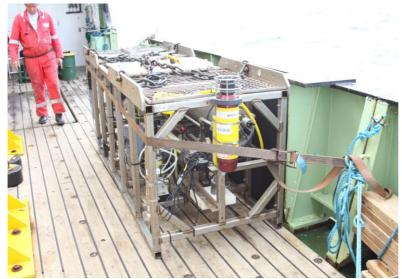
Figure 89. SHRIMP showing the mounting of the USBL system.
