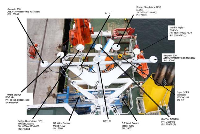
Figure 65. Pre 2011 set-up. The only difference is the Spotbeam has now been replaced by the CNAV antenna which occupy s the same position.
