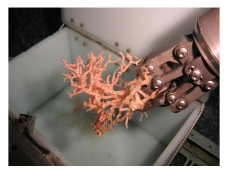
Figure 29. Orion arm being used to place sponge / zoanthid colony into port lidded-biobox.
