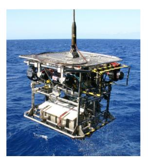
Figure 115. HyBIS vehicle with grab module.
