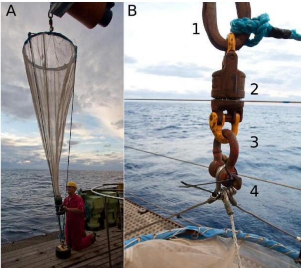
Figure 25. (A) Small ring net rigging overview. (B) Detail of connection between the towing wire (1) and the three-point bridle (4) using a hammerlock swivel (2) and a lifting shackle (3).
