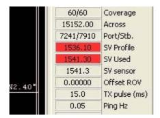
During transits the SVP values in SIS would go red to indicate that the SVP is no longer valid based on data acquired from the hull mounted SVP.
