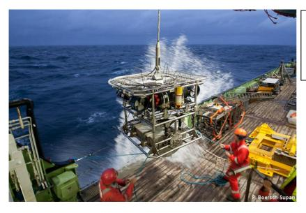
Figure 9. HYBIS towed camera and grab system being recovered on James Cook Cruise JC055. Photograph © Philipp Boersch-Supan.
