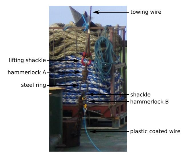
Figure 24. Detail of rigging assembly of the large ring net.
