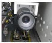
Fig. 5: Forward looking HD camera with laser array
