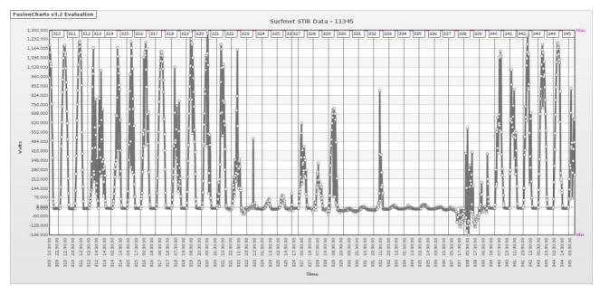
Figure 95. Graph showing issues with windsonic sensor.
