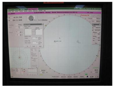
Figure 87. HPR positions displayed on the DP.
