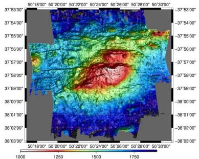
Figure 17. Bathymetry of Middle of What Seamount from current cruise (2011) data
