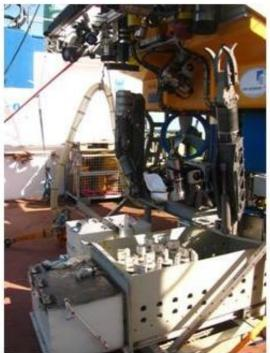
Fig. 2a: ROV KIEL 6000 with Configuration 1: port drawer with 16 pushcores and lidded biobox in front; starboard drawer with 2 lidded bioboxes.
