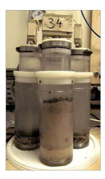
Figure 44. An example of a good, quantitative ROV push core (front) with two examples of poor cores, suitable only for use as qualitative samples, on either side.
