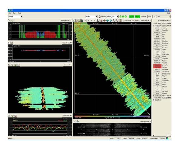
Figure 72. On one occasion during the cruise a problem occurred where no centre beam data was displayed in SIS. Stopping and restarting SIS solved this issue. During this stage we did not have an accurate sound speed profile.
