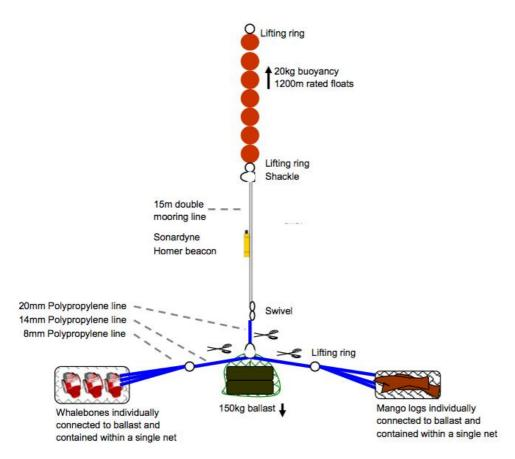
Figure 45. Mooring schematic. The scissor symbol designates where the ROV should cut during recovery.
