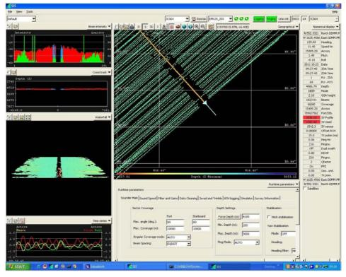
Figure 73. A similar issue occurred with a visible raised area below the vessel. As with the "no data" problem described above, this was solved restarting SIS.
