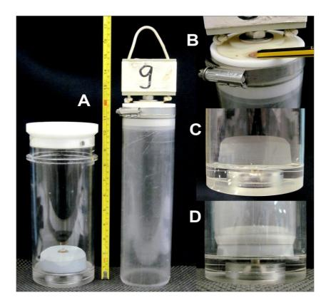
Figure 43. Design of the *Kiel* 6000 Push Core system. A: Complete system showing quiver on the left and core on the right, B: Detail of top insert showing silicone flap valve, C: Detail of base of quiver showing fixed sealing bung, D: Detail of push core seated on sealing bung.
