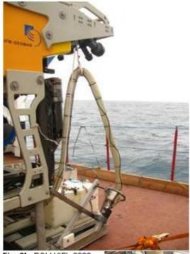
Fig. 2b: ROV KIEL 6000 with Configuration 1: slurp gun nozzle, with attached temperature probe (see right)
