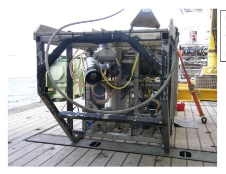
Figure 8. SHRIMP (Seabed High Resolution Imaging Platform) towed camera system. Photograph © Dr Jane Read, NERC.
