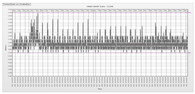
Figure 66. Despite "High Noise" errors on the DP system the actual HDOP values for the DPS116 were very good for the duration of the cruise.
