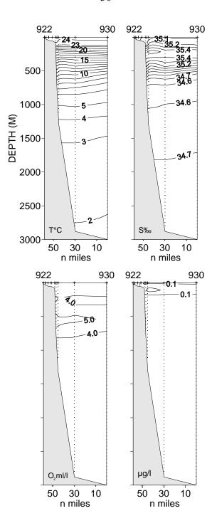
Fig. 3.12. Vertical sections of temperature, salinity, oxygen and fluorescence
