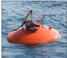
Plate 3. LOCO mooring showing the Floatec buoy with upward looking ADCP
