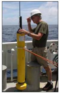
Plate 2. Argo float ready for deployment
