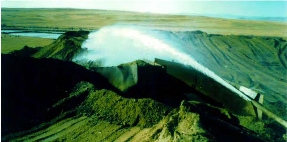
Fig.4: Poor environmental mine management at Ikh Alt Ltd., where an idle water monitor jetting water has been turned towards the tailings mounds, causing gullying and washing of sand and mud into watercourses and ponds. The water is pumped from the Tuul river. The water monitors are frequently left on for extended periods, due to the inherent difficulty of priming water pumps of traditional design when restarting them. This can be overcome by switching to water pumps of modern design. (Photographer: Jeff McCusker, October 1999).
