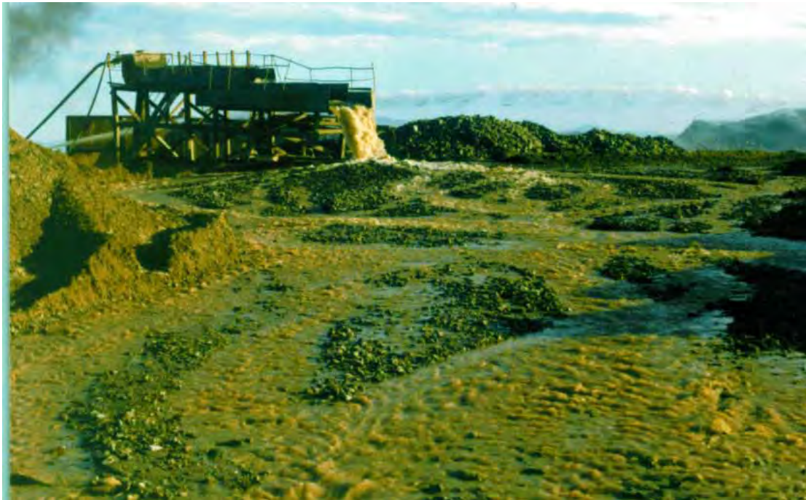
Fig.6: Example of inefficient technology, a traditional style sluice that is incapable of recovering fine gold, and requires excessive use of water, which rapidly fills settling ponds with sediment, and causes inadequately treated waste-water to overflow in an uncontrolled manner due to the large volumes of water used. (Photographer: John Farrington, August 2000).
