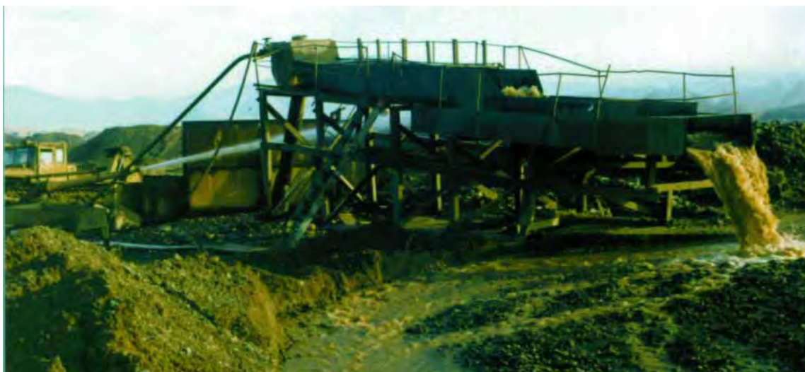
Fig.1: Typical gold recovery system in the Zaamar Goldfield, using old technology with a low % gold recovery rate and large water demand, Shijir Alt Mine of Mongolrosvestmet JSC. (Photographer: John Farrington, August 2000).
