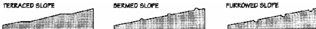
Fig.22: Erosion control on slopes by construction of slope terraces, berms and furrows (from Norman 1997).
