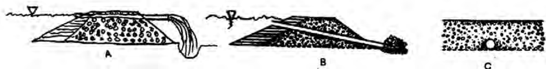
Fig.17: A) Poor settling pond outflow culvert design. Note that clean pond water cascades out of horizontal culvert pipes, sometimes falling up to 3 m, eroding a large hole at the base of the pond dike. B) Cross-section view of a proper settling pond outflow design. Note that the culvert pipe is angled downward through the dam and large rocks and boulders have been placed at the culvert outlet to dissipate flow energy. C) front view of pond dam (from Hanneman 1987).
