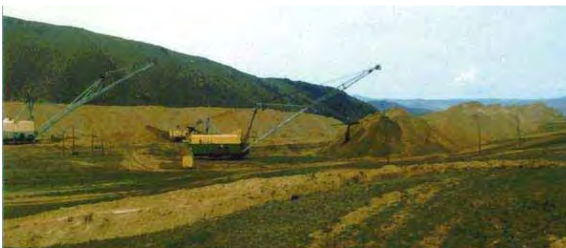
Fig.8: Two drag lines active in the Hailaast Valley, a minor tributary of the Tuul river. Note steep-sided mounds of overburden dumped close to hillside on left. (Photographer: John Farrington, August 2000).
