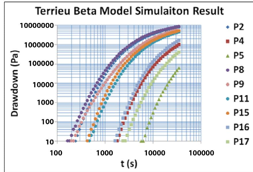
Similar **clustering** behaviour of the pressure curves indicates the flow model can preserve the expected **hierarchical flow behaviour**!
