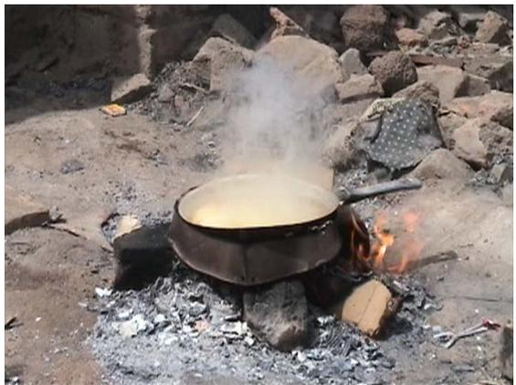
*Gold particles are leached with nitric acid to remove iron oxide crusts*
