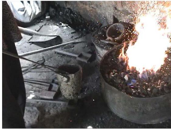
*Gold “cleaned” with nitric acid is melted with borax*
