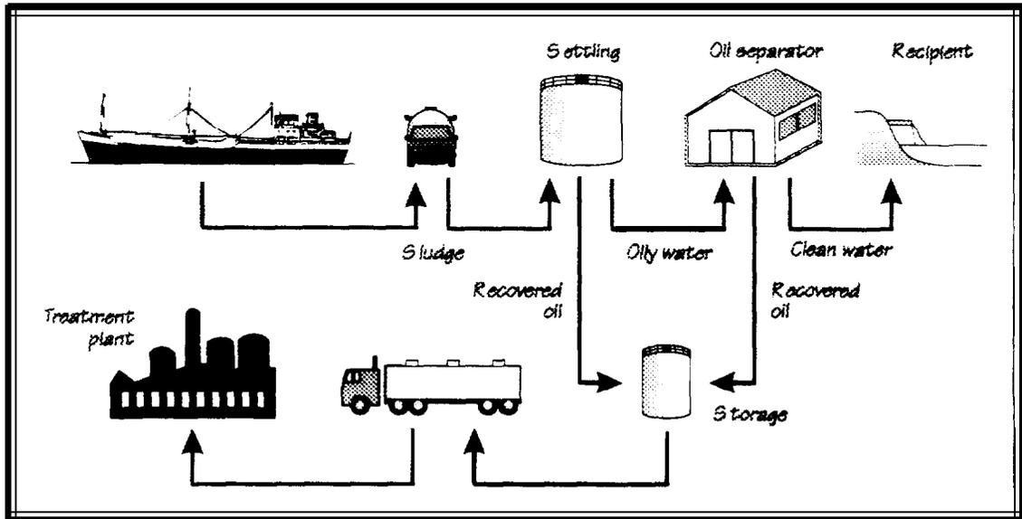
Fig. 1. Engine room wastes from the ship to final processing
