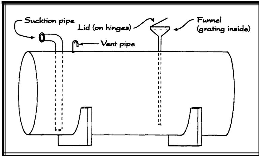
Fig. II. Sketch of tank for a few cubic metres of oily wastes
