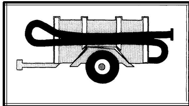
Fig. 2. Small mobile tank for the reception of sludge
