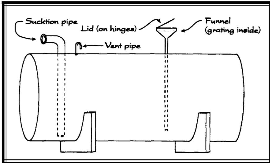
Fig. 11. Sketch of tank for a few cubic metres of oily wastes
