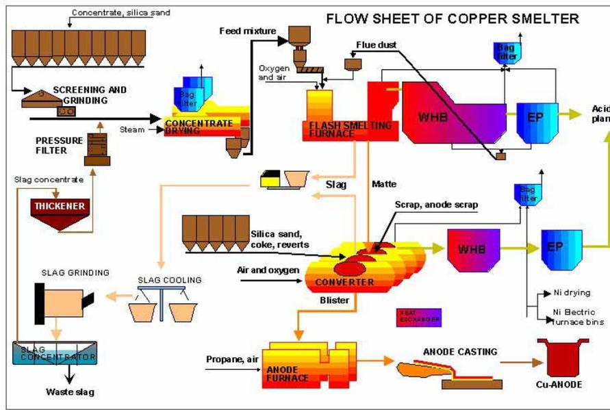
Figure 2. Flow chart for copper smelter at Harjavalta
