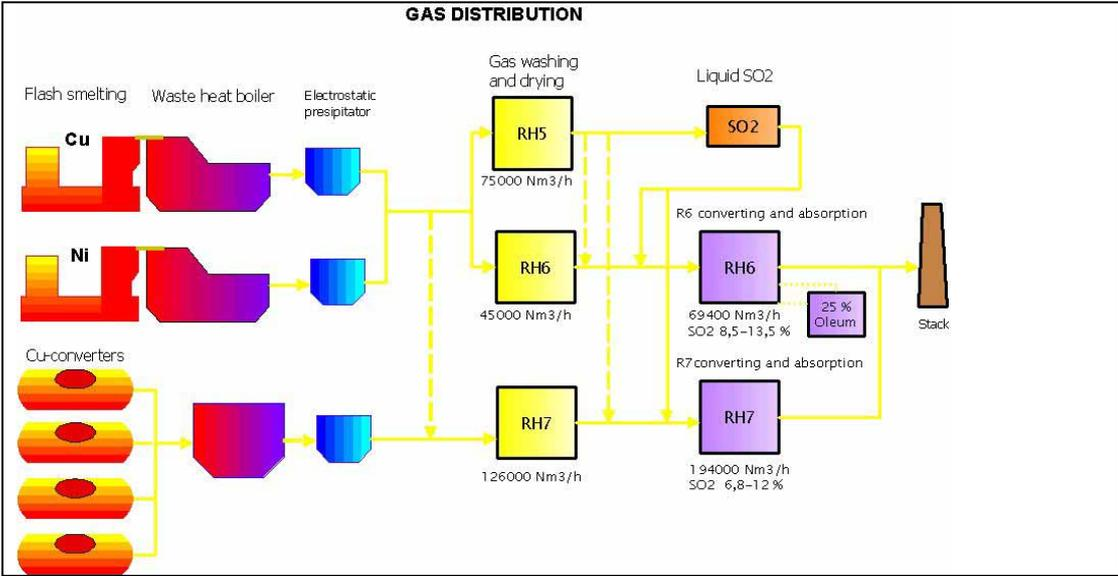
Figure 4. Flow chart for sulphuric acid plant at Harjavalta
