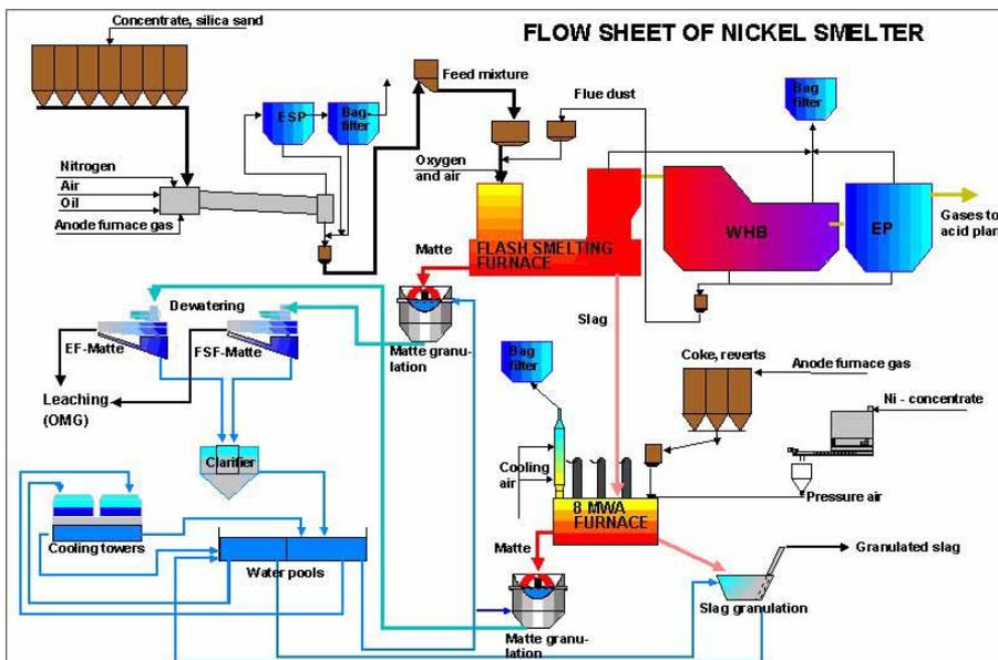
Figure 3. Flow chart for nickel smelter at Harjavalta
