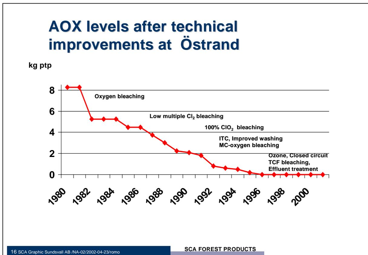
Oxygen bleaching was established at the mill from as early as 1982. In 1986 environmental research revealed that kraft pulp bleaching was one of the most significant sources of dioxin emissions. As a result, low multiple chlorine bleaching was introduced in the late eighties to help eliminate the release of dioxins. AOX emissions were reduced to approximately 2 kg per ton of pulp.
