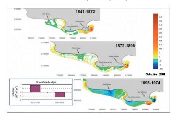
Figure 3. Sedimentary losses (1895 to 1974/88) on the upper shoreface (0-20 m). Bathymetric comparison and shore face budget.
