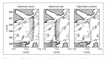
Figure 1. Typical examples of the depth-averaged tidal and mean currents in the Marsdiep inlet as observed with the ferry-ADCP on the route den Helder-Texel.
