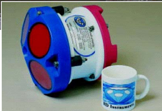
ADCP WORKHORSE RIO GRANDE 1200 kHz (SEBA, RDI-Instrument) Mode 12 (High Resolution, Shallow water profiling in rivers and streams)
