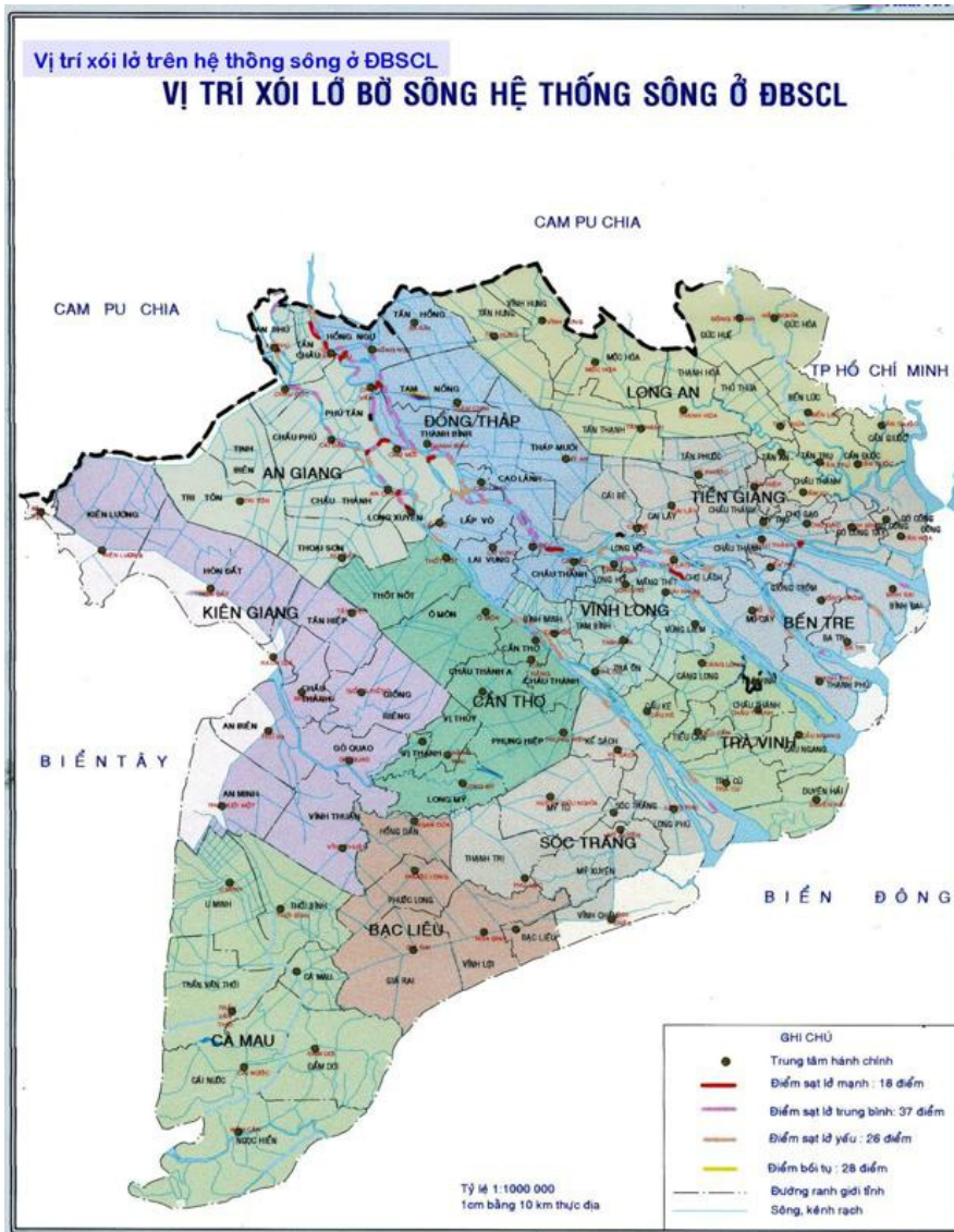
Figure 10: Map of river bank erosion in the Mekong delta. Reaches subject to erosion rate > 10 m/year are in red colour, from 5-10 m/year are in purple and < 5 m/year are in pink. Source: Southern Institute of Water Resources Research
