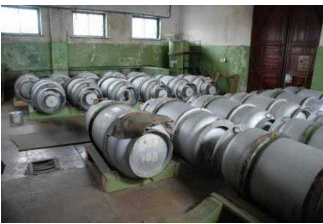
Photo. 6. Storage house of chlorine in containers
