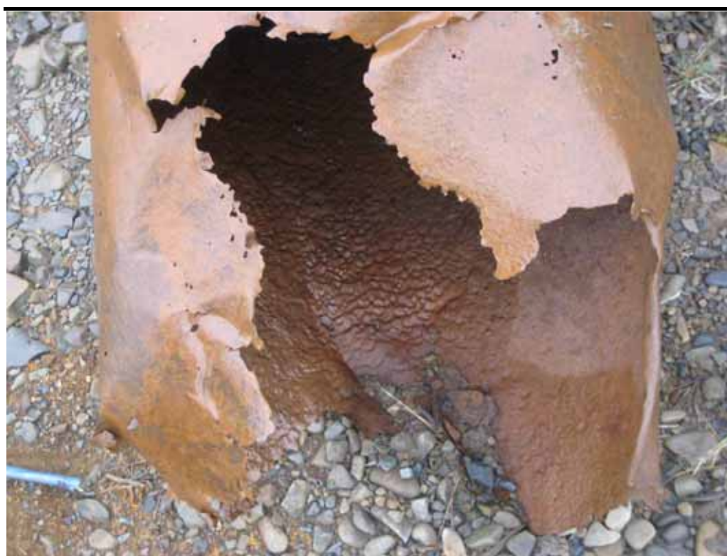
Photo 4 Due to the corrosive medium of the tailings pond, the siphon tube (8mm thick) abstracting water from a depth of 1.2m deteriorates completely within 1.5 to 2 years.
