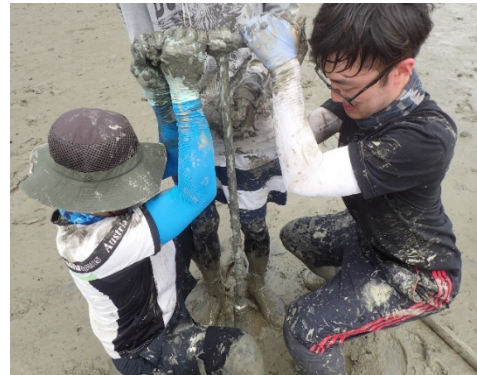
Core sediment sampling
