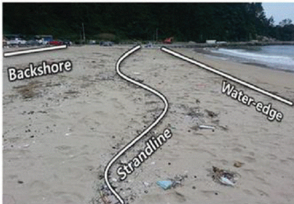
FIG. 4-1 The referent lines for beach sediment sampling (IOC-WESPAC, 2018).
