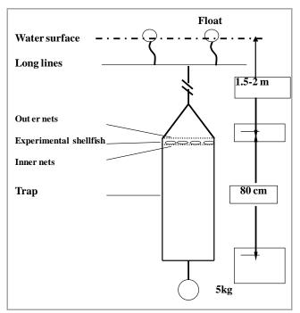
Fig.3 Schematic diagram of the biodeposition trap
