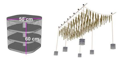
Fig. 3-2 The structure of longline system for abalone-seaweed-sea cucumber integrated aquaculture
