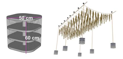
Fig. 3 The structure of longline system for abalone-seaweed-sea cucumber integrated aquaculture
