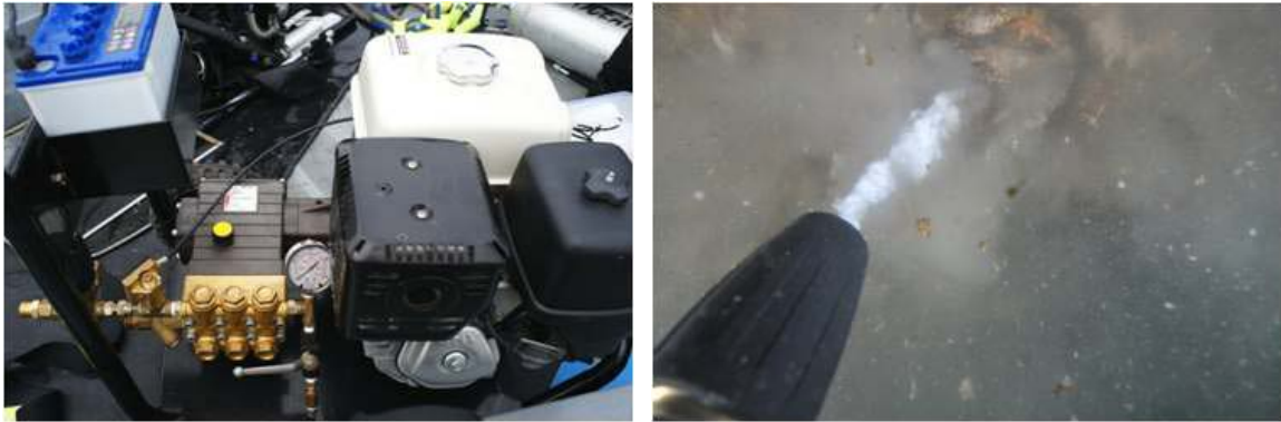
Figure 19. Underwater jet machine and its use in jellyfish polyp removal
