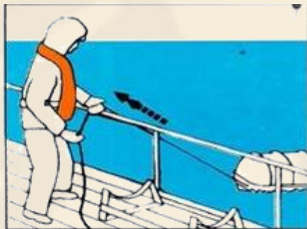
Pull on painter line until it stops and liferaft starts inflating
