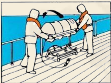
Ensure painter is secured to a strong point then throw liferaft overboard
