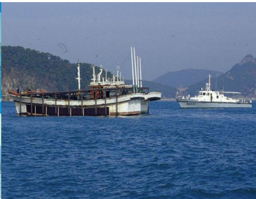
Wooden ship and steel composite AR (3×15×4 m) (50t)
