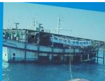
Wooden ship and steel composite AR (3×15×4 m) (50t)
