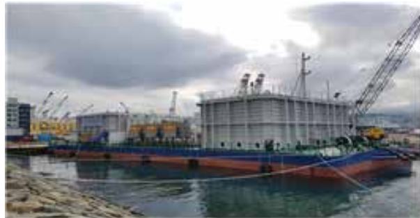
Movable facilities for testing ballast water treatment devices
