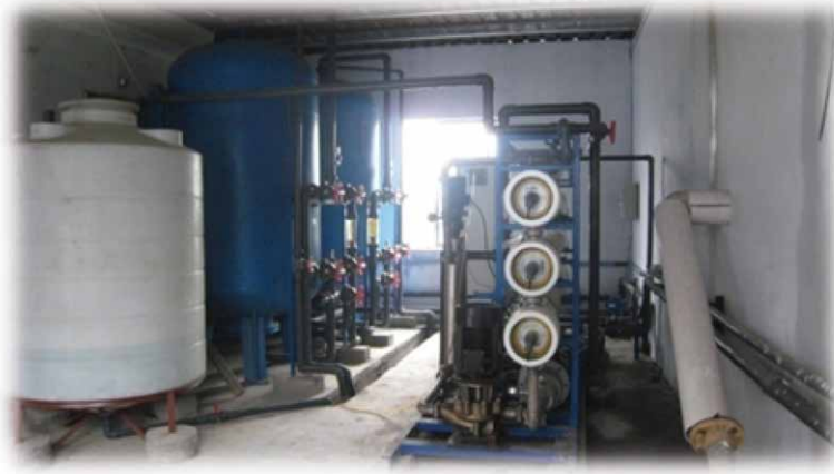
Figure 3-11 Seawater concentrator. (Zhejiang Mariculture Research Institute)
